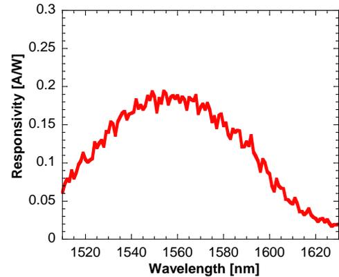
Fig. 5. Wavelength dependence of responsivity measured at 4 V.
