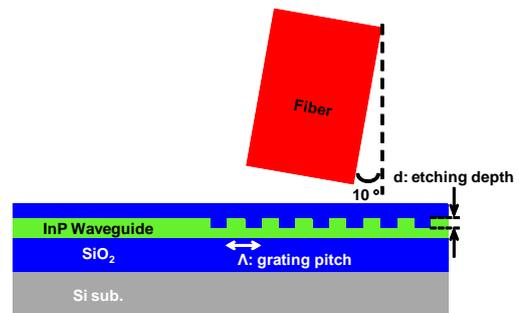
Fig. 2 Schematic of InP grating coupler on III-V-OI wafer
