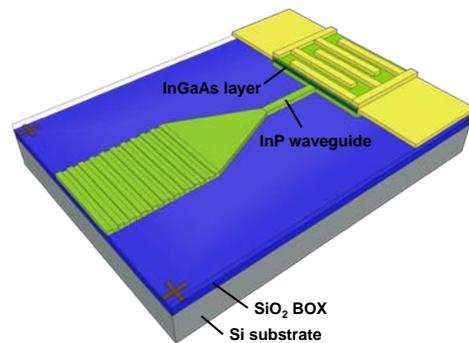
Fig. 1 Schematic of waveguide InGaAs MSM PD with grating coupler on the III-V CMOS photonics platform.
