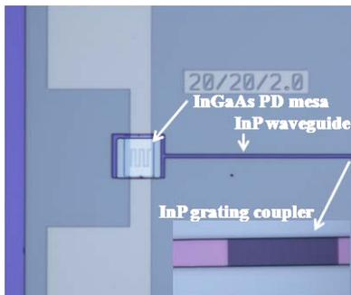
Fig. 4 Plan views of waveguide InGaAs MSM PD integrated with grating coupler.
