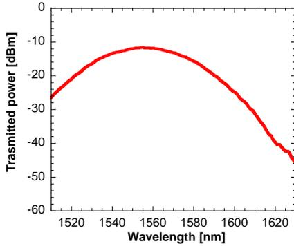
Fig. 3 Measured transmitted power of InP grating coupler on III-V-on-insulator wafer.
