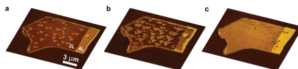
Fig. 1. Atomic force microscopy images of bilayer and 4-layer WSe 2 on SiO 2 after O 3 exposure at 70 °C for (a) 0.5, (b) 1, and (c) 1.5 hours.
