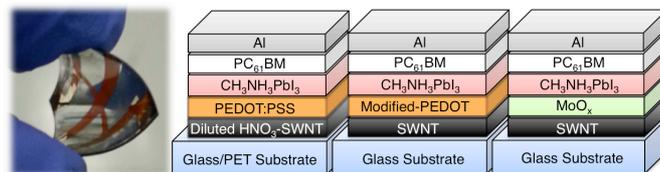
Fig. 1 A picture of flexible application (left) and illustrations of various structures (right)
