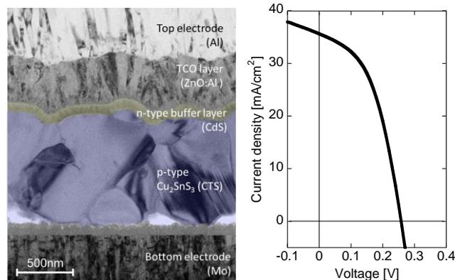
Fig. 2 Typical structure (left) and  $J$ - $V$  characteristics (right) of a CTS cell showing 4.29% efficiency.
