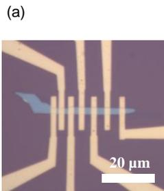
Fig. 5 (a) Optical image showing an array of MoS<sub>2</sub> FETs with Ni-graphene electrodes. The channel lengths varying from 0.5 to 3  $\mu$ m, in steps of 0.5  $\mu$ m. (b)  $R_C$  as a function of  $V_G$ . The  $R_C$  reported by others for MoS<sub>2</sub> FETs are included for comparison.
