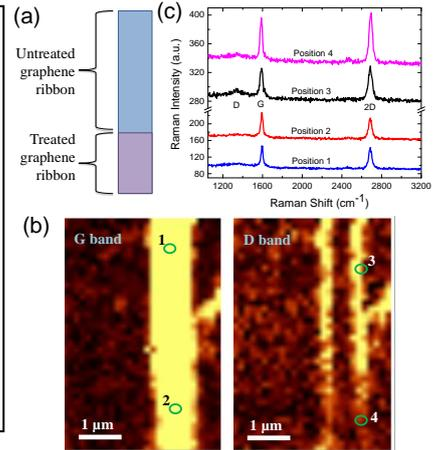
Fig. 3 (a) Schematic of a graphene ribbon defined by oxygen plasma and then partially treated with Ni-mediated etching. (b) Raman maps showing the intensity of the G- and D-band of the partially treated graphene ribbon. (c) Raman spectrum taken at the positions indicated in b.
