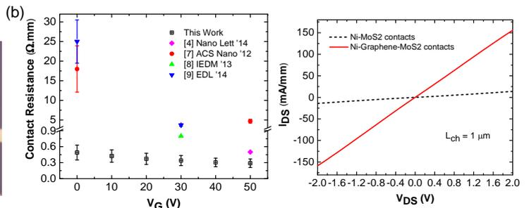
Fig. 6  $I_D$ - $V_D$  characteristics of MoS<sub>2</sub> FETs with and without the treated graphene as a contact interlayer ( $V_G = 50$  V).
