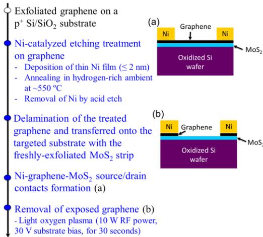
Fig. 1 Top-down process flow to fabricate MoS<sub>2</sub> FETs with Ni-graphene electrodes. Schematics of the device structure (a) prior to and (b) after the removal of exposed graphene on the effective channel regime.
