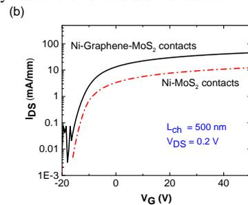
Fig. 7 Comparison of  $I_D$ - $V_G$  characteristics for both MoS<sub>2</sub> FETs with and without the treated graphene as a contact interlayer that were fabricated on the same MoS<sub>2</sub> flake in (a) linear and (b) logarithmic scale.
