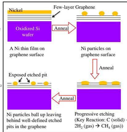
Fig. 2 Schematics illustrating the formation of well-defined etched pits in the few-layer graphene by the proposed Ni-catalyzed etching treatment.
