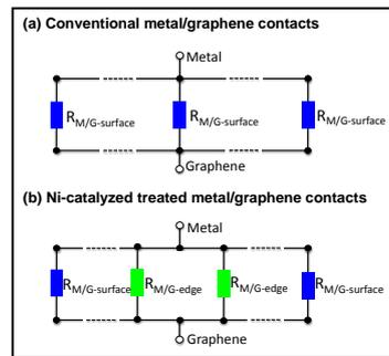
Fig. 4 Resistor network models comparison. It should be noted that  $R_{M/G-edge} \ll R_{M/G-surface}$ .
