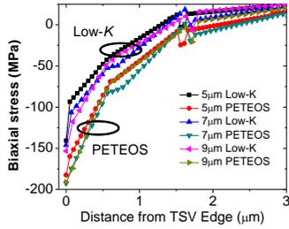
**Fig. 3.** (FEA Simulation) Thermo-mechanical stress exerted by a single Cu-TSV on Si as a function of distance from the edge of TSV.
