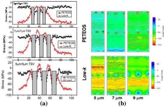
**Fig. 4.** (a) Si Stress profile (biaxial) along TSV rows from Raman Measurement ( $\lambda = 488$  nm). Each row contains 3 TSV with similar TSV pitch and diameter (5, 7, 9  $\mu\text{m}$ ). The stress profiles show that low-k liner is more compliant and can cushion stress exerted by Cu-TSV on the Si (between TSV) more effectively than PETEOS oxide; (b) Biaxial stress mapping of the Si based on micro-Raman spectroscopy.
