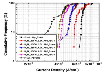
**Fig. 6.** IV measurement of  $\text{Al}_2\text{O}_3/\text{low-}k$  bi-layer liner after annealing. Leakage current density is improved to a level comparable with PETEOS oxide liner after annealing in forming gas ( $\text{N}_2/\text{H}_2$ ) at 350 °C for 2 hours or at 400 °C for 0.5 hour.
