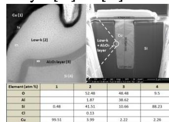
Fig. 2. FIB image of TSV and TEM close-up view of the liner stack.
