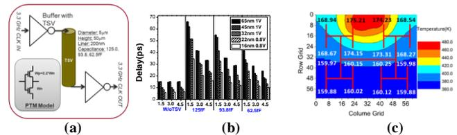
Fig.1. (a) TSV signal delay estimation using predictive technology model (PTM) for different capacitance; (b) Comparison of TSV signal delay for different technology node, *n*-MOSFET width ( $W_n$  in  $\mu\text{m}$ ) and TSV capacitance (fF); (c) H-tree clock skew (ps) due to non-uniform hot-spot heating and the corresponding spatial variation in TSV capacitance.
