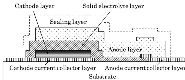
Fig. 1. Schematic drawing of TFB.
