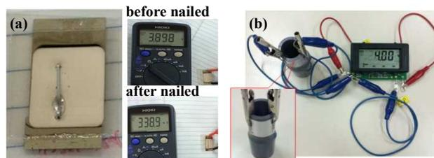
Fig.4. Appearance of reliability test; (a) Nailing test, (b) LCD driving test by bended battery.
