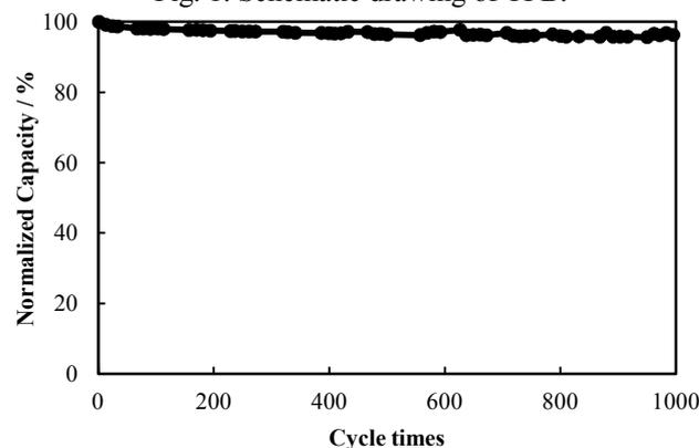
Fig. 2. Charge/discharge cycle performance of TFB.
