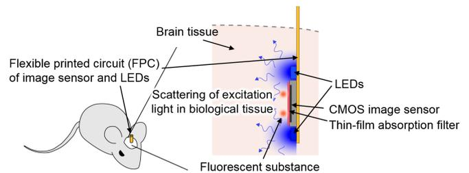
Fig. 1. Schematics of lensless fluorescence imaging of mouse brain using a needle-like shaped imaging device. (a) The imaging device is inserted into a brain tissue. A flexible printed circuit (FPC) can be connected to a personal computer (PC). (b) Brain tissue is illuminated by implanted LEDs and fluorescent images can be obtained by the CMOS image sensor with thin-film absorption filter.
