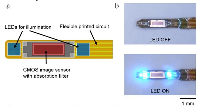
Fig. 2. Schematics and photographs of needle-like shaped imaging devices. (a) The imaging device is constructed with the CMOS image sensor chip with 450- $\mu\text{m}$ -width, 1500- $\mu\text{m}$ -length, and 150- $\mu\text{m}$ -thickness and the LEDs with 280- $\mu\text{m}$ -width, 305- $\mu\text{m}$ -length, and 90- $\mu\text{m}$ -thickness, and the flexible printed circuit (FPC). (b) The LEDs for illumination was mounted beside the CMOS image sensor chip.
