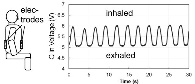
Fig. 1: The hand-made capacitance sensor signal using the electrodes (conductive textile of DW-372N) at the abdomen and backside. The output voltage increases when the capacitance increases.
