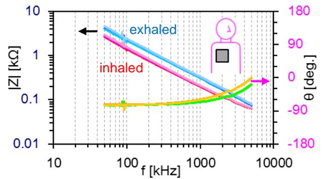
Fig. 5: Frequency response of the signal. The electrodes are pasted on the right chest and its back. The shielding cover wear is also found to be effective for stabilizing the signal.
