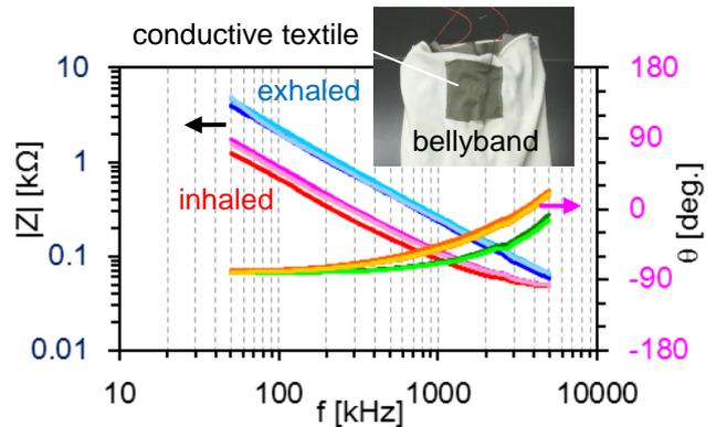
Fig. 6: Signals when the electrodes are fit on the chest center and its back using the bellyband with the shielding cover.
