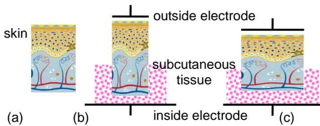
Fig. 3: (a) Typical skin structure. The model of the electrodes consisting the capacitance across the skin at (b) the exhaled and (c) the inhaled conditions.
