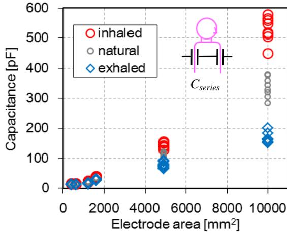
Fig. 4: The capacitance as the function of the electrode area. Two electrodes are pasted on the abdomen. The measurement frequency is 700kHz.
