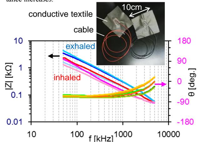
Fig. 2: Typical frequency response of the sensor signal. The electrodes are pasted on the chest center. The response is almost same when the electrode is pasted on the abdomen. The applied voltage amplitude for sensing is 1V.
