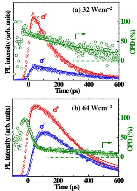
Fig. 1 Circularly polarized transient PL and the corresponding CPD in InGaAs QDs coupled with an InGaAs QW and a 4 nm-thick barrier of GaAs as a function of excitation power (a: 32  $\text{Wcm}^{-2}$ , b: 64  $\text{Wcm}^{-2}$ ). Solid lines are rate-equation calculations.
