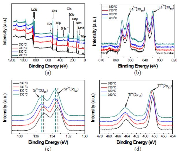
**Figure 3.** X-ray photoelectron spectra of (a) Survey scans, (b) La 3d, (c) Sr 3d and (d) Ti 2p at different calcinations temperature.
