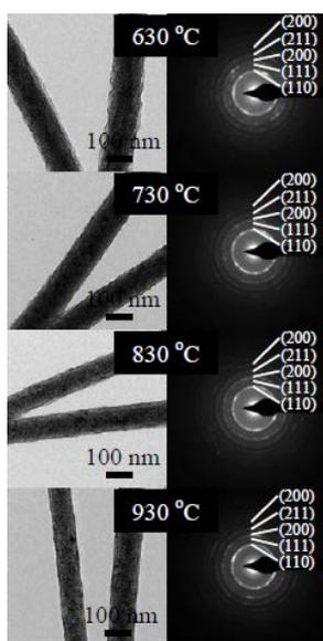
**Figure 1.** TEM bright-field images with corresponding selected-area electron diffraction (SAED) of  $\text{La}_{0.5}\text{Sr}_{0.5}\text{Ti}_{0.95}\text{Co}_{0.05}\text{O}_3$  nanofibers calcined in argon for 2 h at different temperature.
