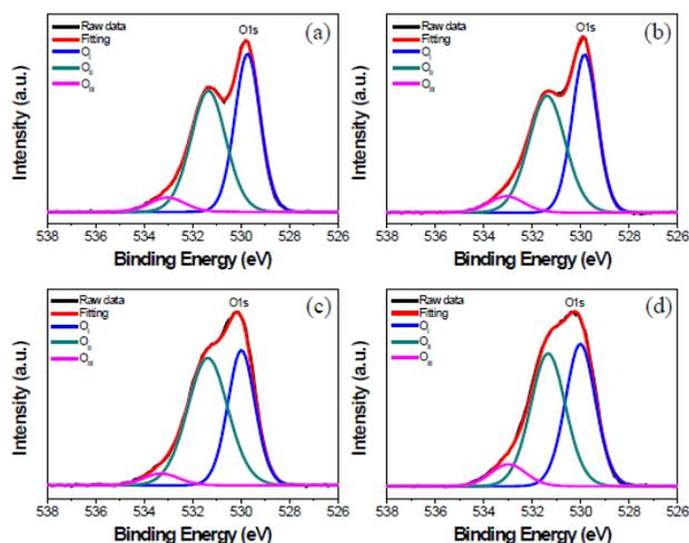
**Figure 4.** XPS profiles of O1s for different calcinations temperature: (a) 630 °C, (b) 730 °C, (c) 830 °C and (d) 930 °C.
