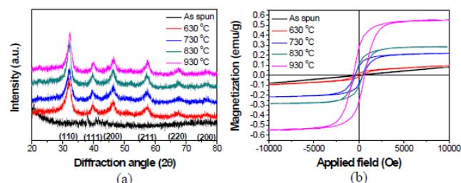
**Figure 2.** (a) XRD patterns and (b) Magnetization at room temperature measured by VSM of as-spun and  $\text{La}_{0.5}\text{Sr}_{0.5}\text{Ti}_{0.95}\text{Co}_{0.05}\text{O}_3$  nanofibers after calcined in argon for 2 h at different temperature.
