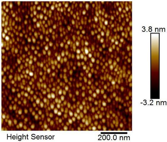
Fig. 1 AFM image of InAs QDs grown on InP(001) 6° off substrate with As<sub>2</sub> flux.
