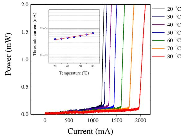
Fig. 3 Temperature dependence of I-L characteristics. Inset: temperature dependence of threshold current.
