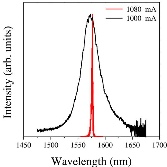
Fig. 2 EL (black line) and laser (red line) spectra of 30-layer stacked QD laser at room temperature. Ground state lasing was obtained at 1576 nm with this laser.
