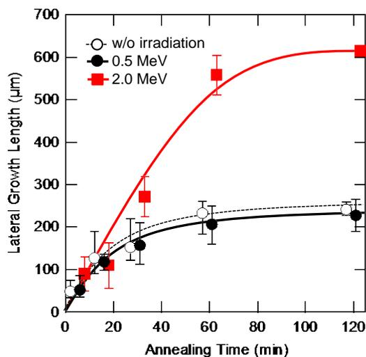
Fig. 3 Annealing time dependence of the lateral growth length of the samples with and without various energy electron irradiations (Electron fluence :  $1 \times 10^{17}$  e/cm<sup>2</sup>).
