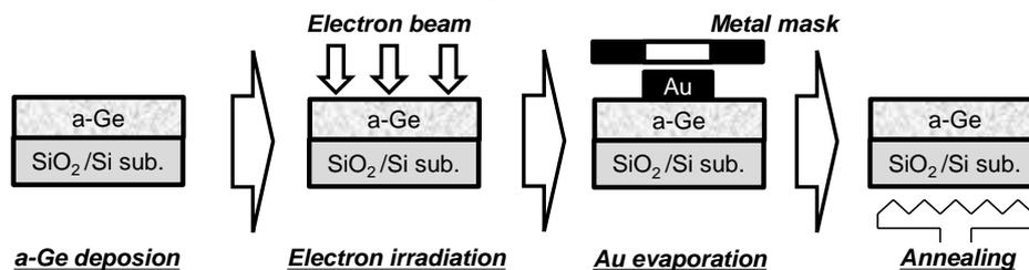
Fig. 1 Experimental procedure.
