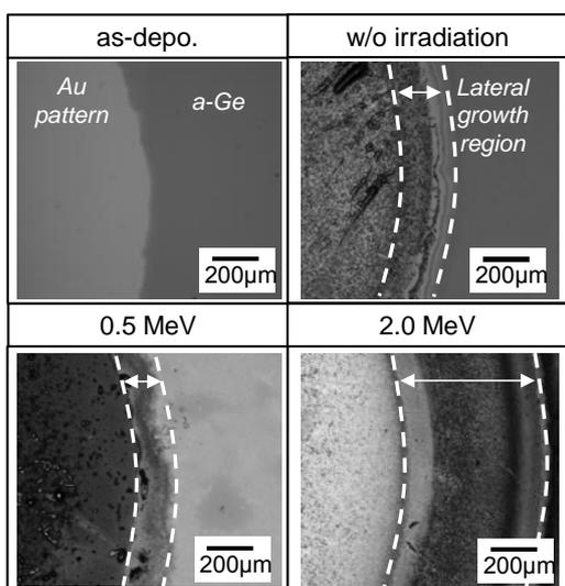
Fig. 2 Nomarski micrographs of the samples with and without various electron irradiation conditions after annealing at 400 °C for 60 min (Electron fluence :  $1 \times 10^{17}$  e/cm<sup>2</sup>).
