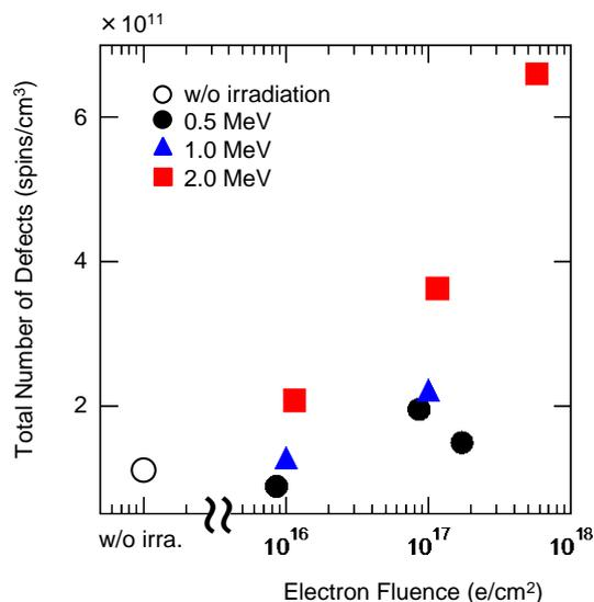
Fig. 5 Electron fluence dependence of total number of defects for the samples with and without various energy electron irradiations.
