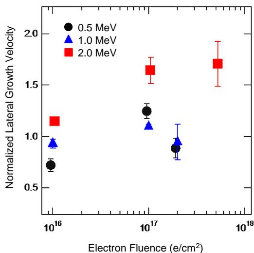
Fig. 4 Electron fluence dependence of normalized lateral growth velocity for the samples with various energy electron irradiations.
