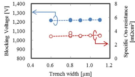
Fig. 6 Trench width dependence on blocking voltage (filled circles) and specific on-resistance (open circles).
