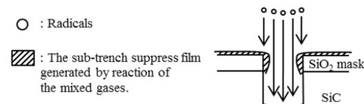
Fig. 2 Schematic of mechanism to suppress sub-trenches.
