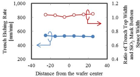
Fig. 3 Wafer uniformity of SiC trench etching rate (filled circles) and dimension ratio of trench top width (open circles).
