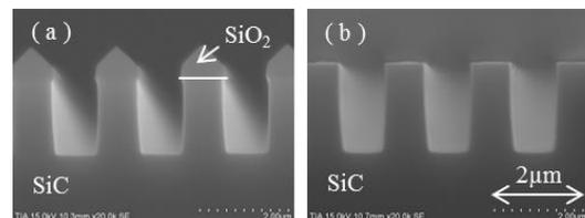
Fig. 1 Cross-sectional SEM images of typical SiC trenches: (a) with SiO<sub>2</sub> mask, (b) without SiO<sub>2</sub> mask (before annealing)
