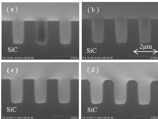
Fig. 4 Cross-sectional SEM images of SiC trenches annealed with solid source: (a) 1350°C, (b) 1400°C, (c) 1500°C, (d) 1605°C.
