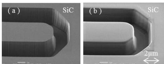
Fig. 5 SEM images of SiC trench before (a) and after (b) the annealing with solid source at 1500°C for reducing surface roughness of the trench sidewalls.
