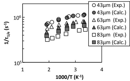
Fig. 3. Temperature dependence of experimental and calculated  $1/\tau_{1/e}$  and for the Si-face of the CMP samples excited by 355 nm
