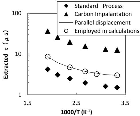
Fig. 2. Temperature dependence of reported  $\tau_{\text{epi}}$ . The line is parallel displacement from the reported dependence with  $\tau_{\text{epi}}$  of 3  $\mu\text{s}$  at room temperature, and the circles are employed values in the calculations.
