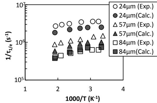
Fig. 4. Temperature dependence of experimental and calculated  $1/\tau_{1/e}$  and for the Si-face of RIE (Si-face) samples excited by 355 nm
