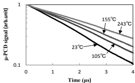
Fig. 1.  $\mu$ -PCD decay curves for the Si-face of the 83  $\mu\text{m}$  thick CMP sample excited by 355 nm
