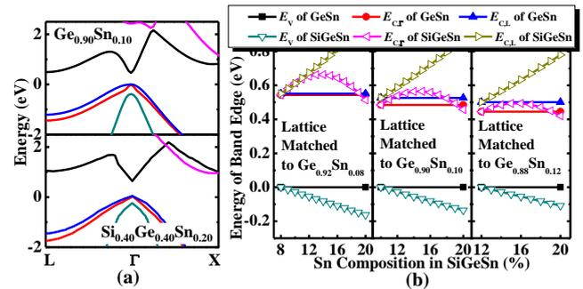
Fig. 1. (a) Energy band structures along L- $\Gamma$ -X direction in the Brillouin zone of  $Ge_{0.90}Sn_{0.10}$  (upper) and  $Si_{0.40}Ge_{0.40}Sn_{0.20}$  (lower) calculated by the nonlocal EPM. (b) Band alignment for lattice matched  $Si_{1-y-z}Ge_ySn_z/Ge_{0.92}Sn_{0.08}$ ,  $Si_{1-y-z}Ge_ySn_z/Ge_{0.90}Sn_{0.10}$ , and  $Si_{1-y-z}Ge_ySn_z/Ge_{0.88}Sn_{0.12}$ . Staggered heterojunction can be formed at Si-GeSn/GeSn interface by increasing Sn composition in SiGeSn.
