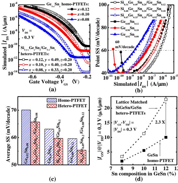
Fig. 3. (a) Simulated  $|I_{DS}|$ - $V_{GS}$  curves for SiGeSn/GeSn hetero-PTFETs and GeSn homo devices. (b) and (c) indicating the superior SS in hetero-PTFETs over the GeSn homo devices. (d) Comparison of  $|I_{ON}|$  for hetero and homo devices with different compositions at  $V_{DD} = -0.3V$ .  $Si_{0.31}Ge_{0.49}Sn_{0.20}/Ge_{0.88}Sn_{0.12}$  hetero-PTFET achieves 2.3 times higher  $|I_{ON}|$  as compared to  $Ge_{0.90}Sn_{0.10}$  homo-PTFET.
