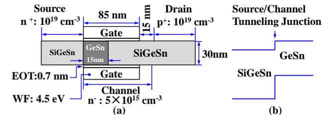
Fig. 2. (a) Schematic of SiGeSn/GeSn hetero-PTFET. (b) Schematic of the type-II staggered tunneling junction at source/channel interface.
