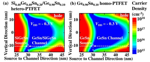
Fig. 5. Contour plots of carrier density for  $Si_{0.40}Ge_{0.40}Sn_{0.20}/Ge_{0.90}Sn_{0.10}$  hetero-PTFET and  $Ge_{0.90}Sn_{0.10}$  homo device at  $V_{DS}=V_{GS}-V_{TH}=-0.3V$ .
