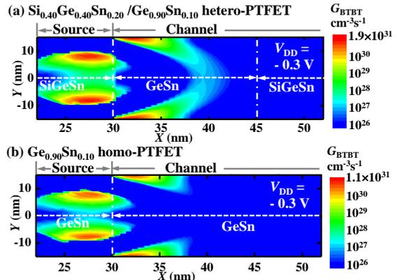
Fig. 6. Spatial distributions of  $G_{BTBT}$  for  $Si_{0.40}Ge_{0.40}Sn_{0.20}/Ge_{0.90}Sn_{0.10}$  hetero-PTFET and  $Ge_{0.90}Sn_{0.10}$  homo device at  $V_{DS}=V_{GS}-V_{TH}=-0.3V$ . The hetero transistor demonstrates a larger peak  $G_{BTBT}$  over homo device.
