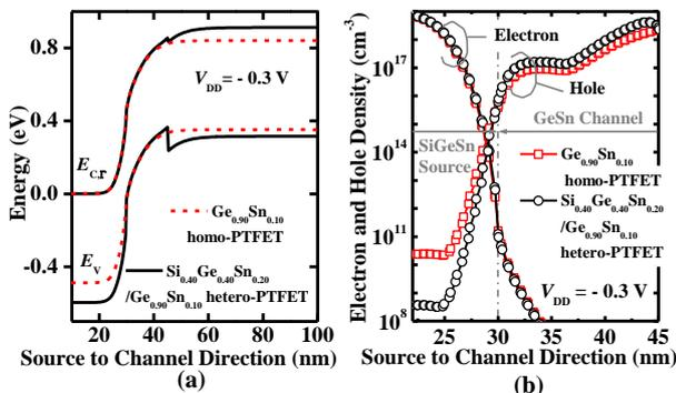
Fig. 4. (a) Energy band diagrams and (b) Carrier density profiles near surface along source to channel direction for  $Si_{0.40}Ge_{0.40}Sn_{0.20}/Ge_{0.90}Sn_{0.10}$  hetero-PTFET and  $Ge_{0.90}Sn_{0.10}$  homo-PTFET at  $|V_{DS}|=|V_{GS}-V_{TH}|=0.3V$ .
