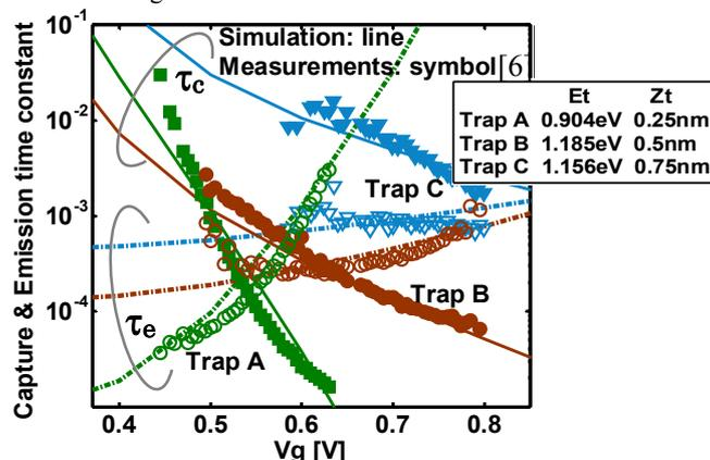
Fig. 2 Dependence of  $\tau_c$  (solid symbol) and  $\tau_e$  (opened symbol) on gate voltage  $V_g$  with three traps. The experimental results[6] is also plotted.
