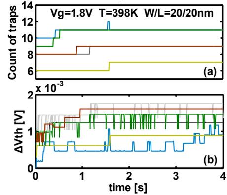
Fig. 6 Degradation of threshold voltage with consideration of traps generation.
