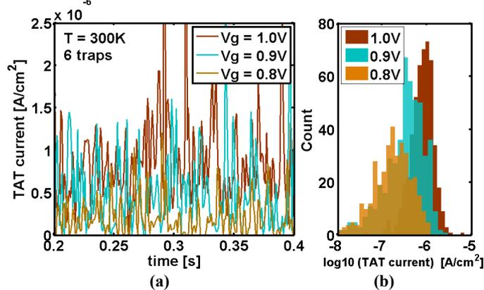
Fig. 5 (a) Transient characteristic of TAT currents with 6 traps corresponding to Fig. 3 under different gate voltage (b) Distribution of Statistical TAT current.
