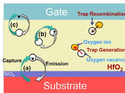
Fig. 1 Multi-physical models including trap generation/ recombination, trapping (a) from/to channel (b) from/to other traps (c) from/to metal gate.
