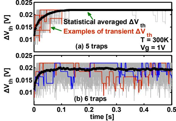
Fig. 4 Transient characteristics of  $\Delta V_{th}$  with (a) 5 traps and (b) 6 traps corresponding to Fig. 3. (black line: statistical averaged  $\Delta V_{th}$ , red/blue line: typical examples of transient  $\Delta V_{th}$ , gray line: 100 samples)
