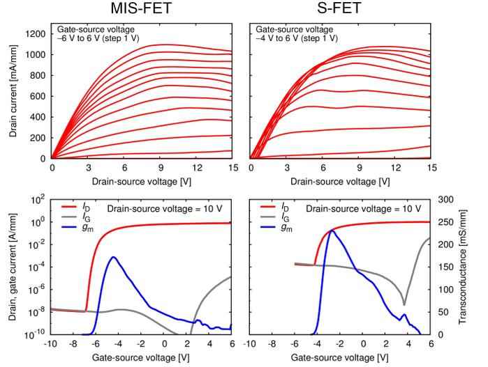
Fig. 1: Output (top) and transfer (bottom) characteristics of the fabricated MIS-FETs and S-FETs.
