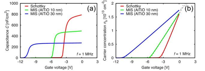
Fig. 2: (a)  $C$ - $V$  characteristics and (b)  $n_s$ - $V$  characteristics of Schottky and MIS capacitors measured at frequency  $f = 1$  MHz.
