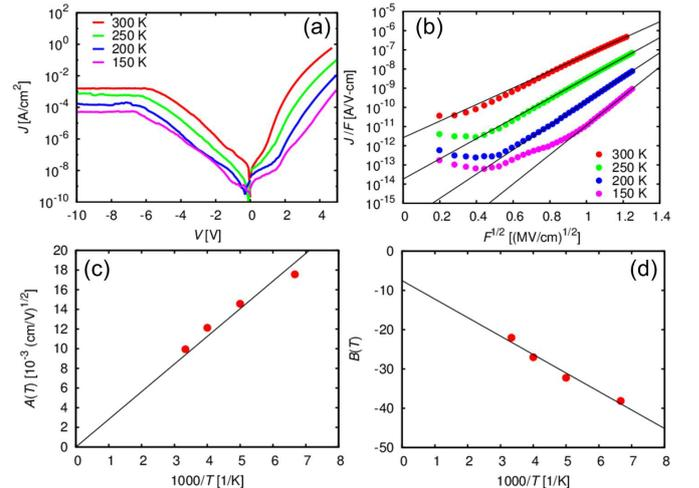
Fig. 3: (a)  $J$ - $V$  characteristics and (b) PF plot of the MIS capacitor for several temperatures. Temperature-dependences of (c)  $A(T)$  and (d)  $B(T)$ .
