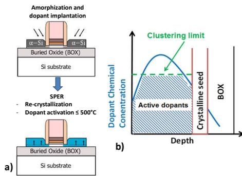
**Fig. 2:** a) SPER mechanism and b) optimization challenges. Seed control; Clusterization phenomenon. Striped areas indicate active dopant regions.
