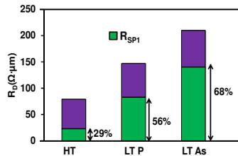
**Fig. 5:**  $R_{SP1}$  contribution extracted by TCAD simulations and percentage of  $R_{SP1}$  on total  $R_{access}$ .
