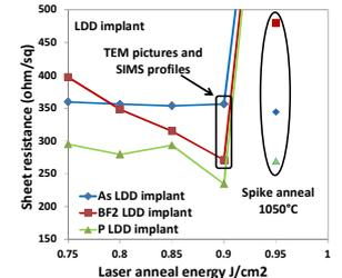
**Fig. 10:** Sheet resistance measurements for As, BF2, P versus laser anneal energy. RTA spike sheet resistance as reference.
