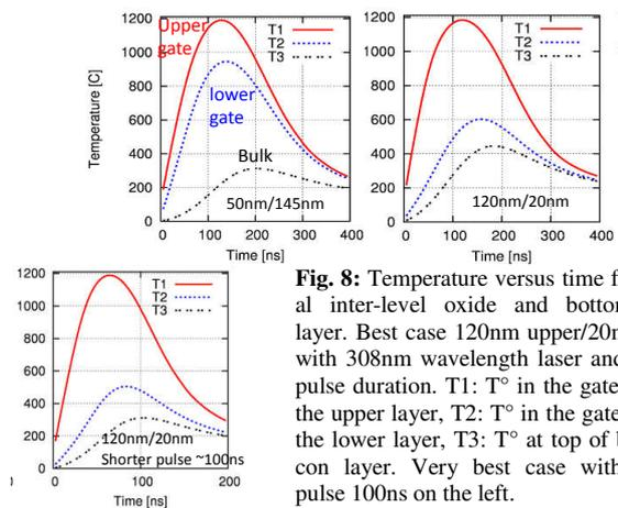
**Fig. 8:** Temperature versus time for several inter-level oxide and bottom oxide layer. Best case 120nm upper/20nm lower with 308nm wavelength laser and ~200ns pulse duration. T1:  $T^{\circ}$  in the gate stack of the upper layer, T2:  $T^{\circ}$  in the gate stack of the lower layer, T3:  $T^{\circ}$  at top of bulk silicon layer. Very best case with shorter pulse 100ns on the left.
