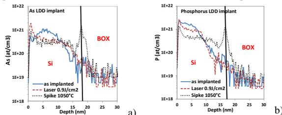
**Fig. 11:** SIMS profiles for a) As b) P LDD implants: as implanted, after laser anneal at  $0.9 \text{ J/cm}^2$  and RTA spike  $1050^{\circ}\text{C}$ .
