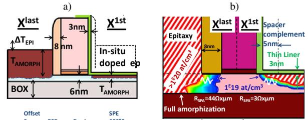
**Fig. 6:** a)  $X^{last}$  and  $X^{1st}$  integration description with process flows. b) KMC simulation of junction profile for  $X^{1st}$  and  $X^{last}$  process flow with SPER.
