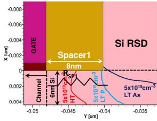
**Fig. 4:** Evolution of Iso-concentration at  $5 \times 10^{19} \text{ at/cm}^3$  for each dopant of Figure 3.
