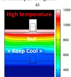
**Fig. 7:** a) Illustration of laser thermal anneal effect on temperature profile b) Optimized 3D simulated structure. SiN 30nm, lower BOX 20nm, inter-level oxide 120nm. Lg 30nm.
