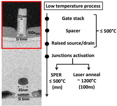
**Fig. 1:** 3DVLSI TEM Cross-section and Low temperature process steps with different types of annealing technique.
