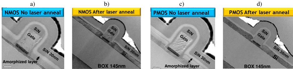
**Fig. 9:** TEM pictures a) as implanted and b) after laser anneal for NMOS planar FDSOI with As implant. c) as implanted and d) after laser anneal for PMOS with BF2 implant.
