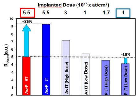
**Fig. 3:** Rsheet measurements for several dopant types and concentrations on 22nm full-sheet implanted SOI wafers. Best condition for LT: low dose Phosphorus.
