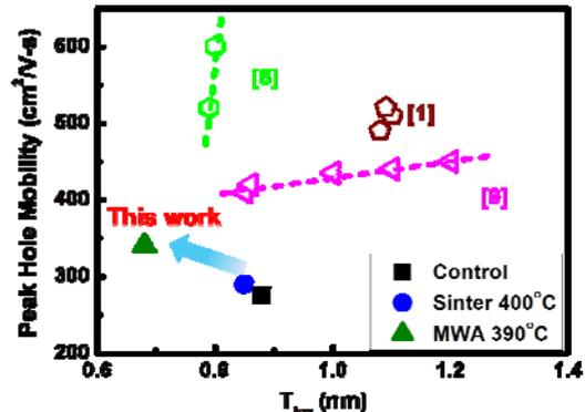
Fig. 6 Peak hole mobility versus T<sub>inv</sub> for Ge pMOSFETs with different process conditions and some benchmarks.
