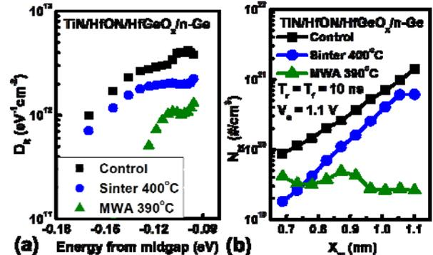
Fig. 4 (a) D<sub>it</sub> and (b) N<sub>bt</sub> at different gate dielectric depths for Ge pMOSFETs in this work.
