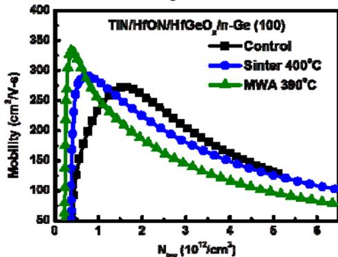
Fig. 5 Hole mobility versus N<sub>inv</sub> for Ge pMOSFETs in this work.
