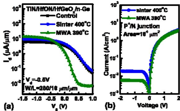
Fig. 3 (a) I<sub>d</sub>-V<sub>g</sub> characteristics of Ge pMOSFETs, and (b) P<sup>+</sup>/N junction characteristics with a sintering and MWA.
