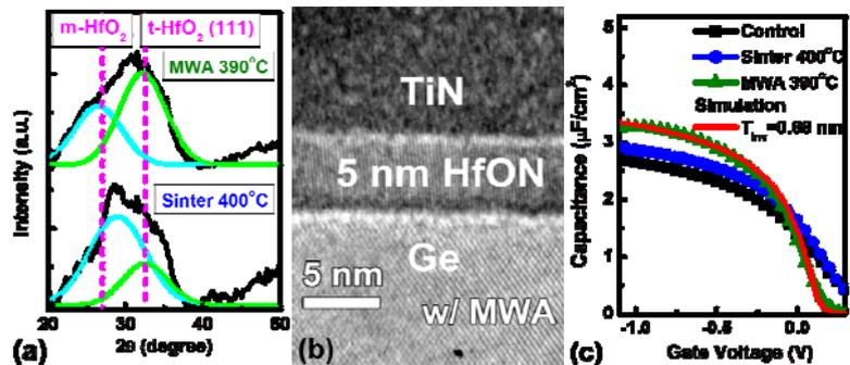
Fig. 1 Cross-sectional view and schematic gate-first process flow of Ge pMOSFETs in this work. Fig. 2 (a) GIXRD spectra of the samples with a sintering and MWA. (b) Cross-sectional TEM image of sample with a MWA and (c) C-V curves for Ge pMOSFETs in this work.
