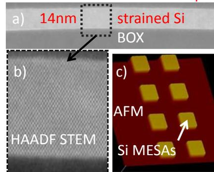
Fig. 5 a-b) Cross-sectional HAADF STEM micrograph of the 14 nm thick Silicon layer after BOX CREEP process. c) AFM mapping of several MESA patterns with no significant roughness.
