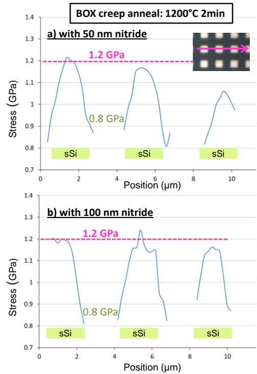
Fig. 4 Stress profiles from 2D Raman extractions for Si MESAs after BOX creep process with a) 50 nm and b) 100 nm thick SiN.
