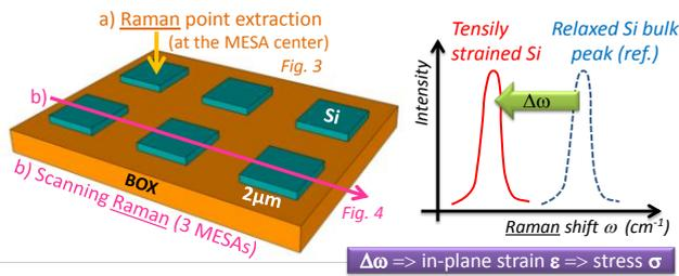
Fig. 2 Schematics of MESA patterns with different Raman measurements and corresponding strain and stress extractions principle.
