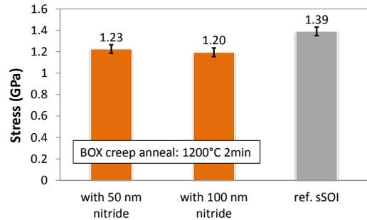
Fig. 3 Average stress calculations from Raman extractions (center of 2x2 μm<sup>2</sup> MESA) for the 14 nm thick Si film of SOI after BOX creep process with 50 nm and 100 nm thick SiN (+sSOI substrate reference). For each sample, 10 sites have been measured.
