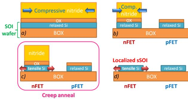
Fig. 1 BOX creep process (starting from SOI wafers) leading to localized sSOI structure for enhanced nFETs: a) SiO<sub>2</sub> and compressive SiN deposition on SOI; b) local SiN etch, MESA patterning; c) creep anneal; d) SiN and SiO<sub>2</sub> layers removal.
