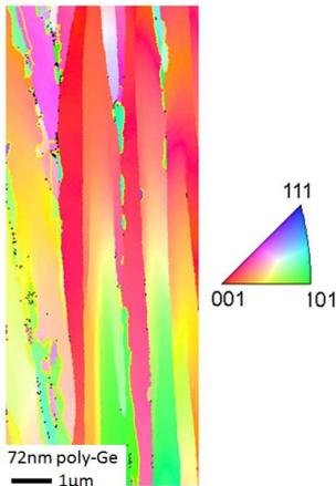
Fig.3 EBSD images of 72-nm-thick P doped ( $5 \times 10^{15} \text{ cm}^{-2}$ ) n-type poly-Ge layer grown by the two-step FLA method.
