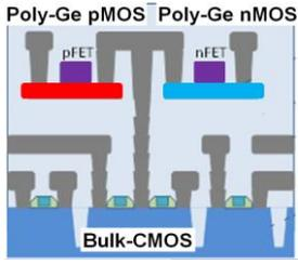
Fig.1 Schematic of monolithic 3D-LSI device formed by sequential stacking of CMOS circuits on underlying CMOS circuits.
