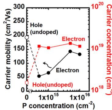
Fig.5 P dose dependence of Hall carrier mobility and the concentration of 72-nm-thick poly-Ge layer grown by two-step FLA method.
