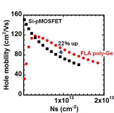
Fig.8 Mobility characteristics for FLA poly-Ge channel tri-gate JL-pMOSFETs obtained by the split C-V method (red circle).
