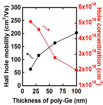
Fig.4 Hole hole mobility and the carrier concentration as a parameter of the FLA poly-Ge thickness.
