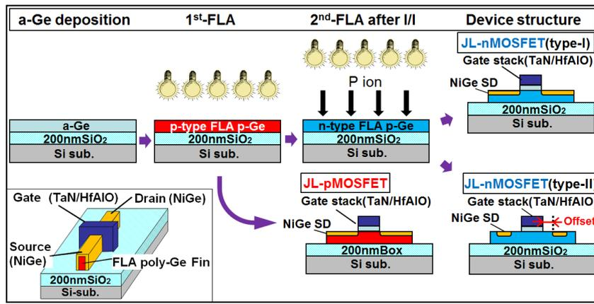
Fig.2 Schematic flow of FLA poly-Ge formation and p and nMOSFETs. Two-step FLA was employed to fabricate junction-less (JL) nMOSFETs. Inset shows schematic structure of the MOSFETs. Two types of SD for nMOSFETs were prepared; Type-I for self-aligned NiGe SD and Type-II for 1.6  $\mu\text{m}$  offset NiGe SD.
