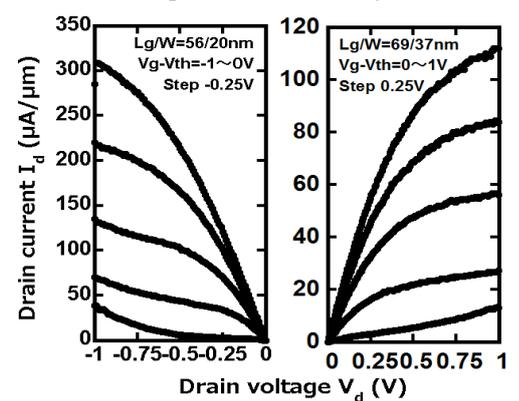
Fig.10  $I_d$ - $V_d$  characteristics of the FLA poly-Ge JL-pMOSFETs ( $L_g/W_{fin}= 56/20\text{nm}$ ) (left) and 2-step FLA poly-Ge JL nMOSFETs ( $L_g/W_{fin}=69/37 \text{ nm}$ ) (right).
