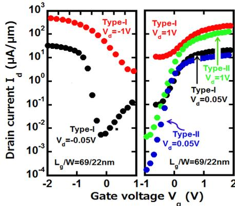
Fig. 9  $I_d$ - $V_g$  characteristics of FLA poly-Ge tri-gate JL pMOSFETs (left) and two-step FLA poly-Ge tri-gate JL nMOSFETs with two types of NiGe SD (Type-I/II) (right). The drain current was normalized by  $2xH_{fin}+W_{fin}$ .
