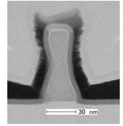
Fig.7 Cross sectional TEM image of a typical n-type two-step FLA poly-Ge fin. Note that the cross section showed no grain boundary.
