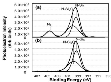
**Fig.1** N 1s XPS spectra for CVD-SiO<sub>2</sub> layers with (a) plasma nitridation only and with (b) plasma nitridation combined with annealing over 900°C, which were taken at a photoelectron take-off angle of 90°. The thickness of CVD-SiO<sub>2</sub> was 10 nm.
