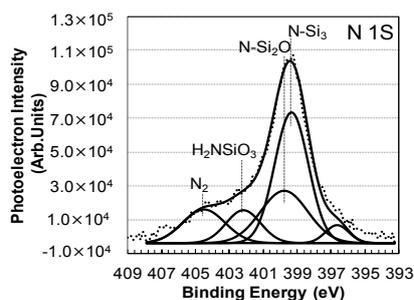
**Fig. 5** N1s XPS spectrum for plasma nitrided CVD-SiO<sub>2</sub> film with subsequent oxide deposition using O<sub>3</sub>-oxidant below 350°C. The photoelectron take-off angle was set at 90°.
