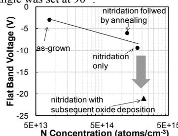
**Fig.8** Flat band voltage of capacitor as function of N concentration in CVD-SiO<sub>2</sub> layer which is determined by SIMS measurement.
