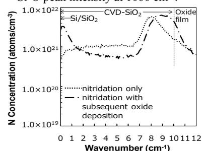
**Fig.6** Depth profiles of N in CVD-SiO<sub>2</sub> layers with plasma nitridation only and plasma nitridation combined with oxide deposition using O<sub>3</sub>-oxidant below 350°C.
