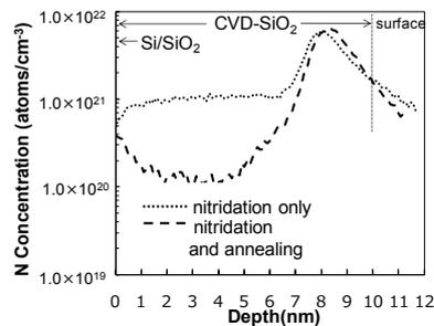
**Fig.2** Depth profiles of N in CVD-SiO<sub>2</sub> layers with plasma nitridation only and with plasma nitridation combined with annealing over 900°C.
