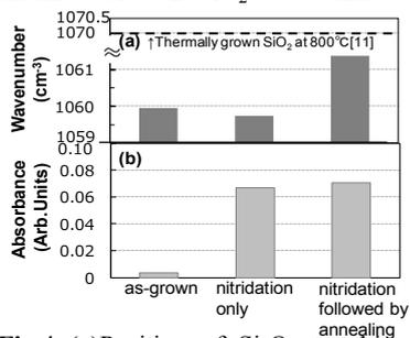
**Fig.4** (a) Position of Si-O stretching vibration and (b) adsorption intensity at 920 cm<sup>-1</sup> for CVD-SiO<sub>2</sub> layers with no additional process, with plasma nitriding only, and with plasma nitridation combined with annealing over 900°C.
