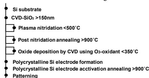
**Fig.7** Process flow for polycrystalline-Si gate MOS capacitors.
