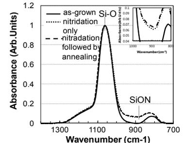
**Fig.3** IR spectra for CVD-SiO<sub>2</sub> layers with no additional process, with plasma nitridation only, with plasma nitridation combined with annealing over 900°C. Each spectrum was normalized with the Si-O peak intensity at 1060 cm<sup>-1</sup>.
