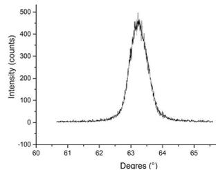
Fig. 7: HR-XRD  $\omega$ -2 $\theta$  scan of the final InGaAs-OI layer.
