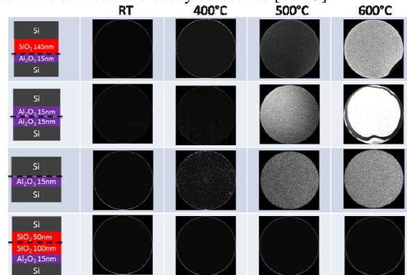
Fig. 9: SAM images of the bonding interface quality for different bonding configurations vs post bonding annealing
