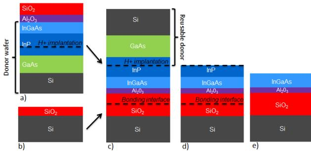
Fig. 4 Fabrication process flow of the InGaAs-OI wafers using the Smart Cut™ technology.
