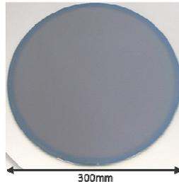
Fig. 5: Picture of the InGaAs-OI after layer transfer
