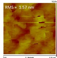
Fig. 2: 5x5 μm<sup>2</sup> AFM scan of the 54 nm-thick In<sub>0.53</sub>Ga<sub>0.47</sub>As.
