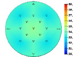
Fig. 3: InGaAs thickness mapping across the 300 mm wafer. Avg. = 54.1 nm. 3σ = 1.7 nm.
