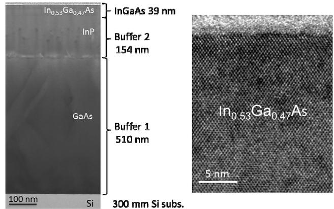
Fig. 1: TEM image of the complete III-V epitaxial stack and HR-TEM on InGaAs channel
