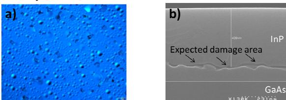
Fig. 8: a) Optical microscope images of the InP surface after H<sup>+</sup> implantation and 300°C annealing b) corresponding SEM image
