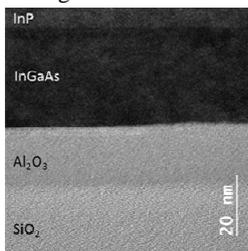
Fig. 6: TEM of the InGaAs-OI after layer transfer.
