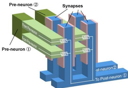
Fig. 7 Schematic of 3D vertical ReRAM array architecture to immunize resistance variation during synaptic training process. The devices with the same pillar electrode can be viewed as a synapse. More devices can be introduced as a combined synapse by increasing horizontal layers.
