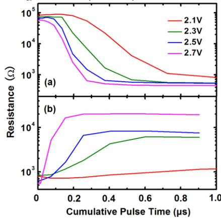
Fig. 4 Measured resistance as a function of cumulative pulse time for TiN/Gd:HfOx/Pt ReRAM device during (a) set and (b) reset process. Multilevel synaptic training processes are observed. Different amplitudes of pulses are used. Training speed increases with pulse amplitude.
