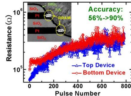
Fig. 8 Measured training process of the top and bottom ReRAM devices in the 3D vertical array by applying 800 identical consecutive pulses. Pulses applied on the two devices with the same vertical electrode at the same time. Inset: TEM image of the fabricated 3D vertical ReRAM cells.
