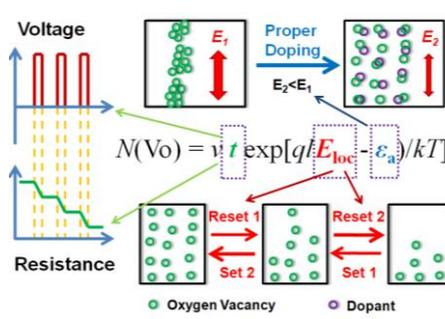
Fig. 2 Schematics of methodology to achieve controlled oxygen vacancy distribution and multilevel switching behavior based on defect engineering. Innovative cell design and operation scheme implementation are developed.
