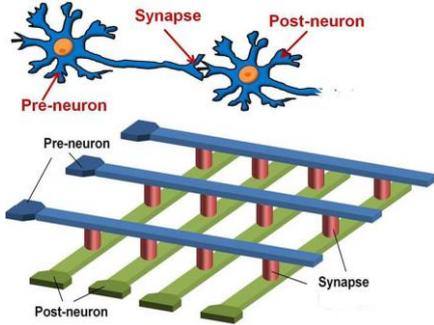
Fig. 1 Schematic view of neural network and TMO-ReRAM based artificial neural network. A neural network is consisted of neurons and synapses. ReRAM array works as synapses to modify the connect strength between pre- and post- neurons.
