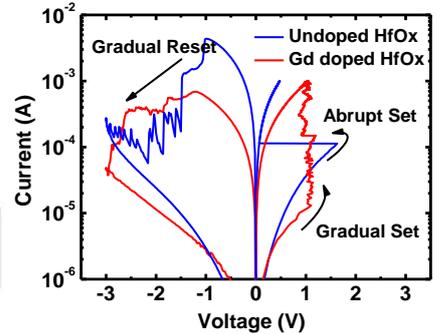
Fig. 3 Typical resistive switching I-V curve of TMO-ReRAM cell before and after optimization. For undoped HfO<sub>x</sub> device, abrupt set process is observed. Whereas, after optimization by doping, multilevel set and reset processes are both easy to realize.
