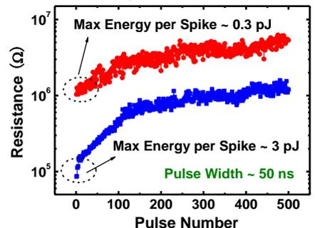
Fig. 9 Measured training process for the fabricated 3D vertical synaptic device with different initial resistance states achieved by different current compliances during the previous set cycles. If starting at 1 MΩ, the maximum energy consumption per spike drops below 1 pJ.
