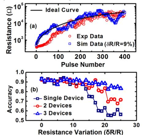
Fig. 6 (a) Measured and simulated multilevel reset training process by 400 identical consecutive pulses. (b) Simulated pattern recognition accuracy of the visual system by paralleling several TMO-ReRAM devices working as a synapse together. A significant improvement is observed as the device number increasing.
