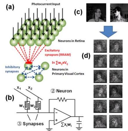
Fig. 5 (a) Schematic of a neuromorphic visual system consisting of two layers of neurons. (b) An implementation of neuron circuit with TMO-ReRAM synapses. (c) Training samples used in the visual system. (d) Simulated final resistance maps of TMO-ReRAM with each cortex neuron after training.
