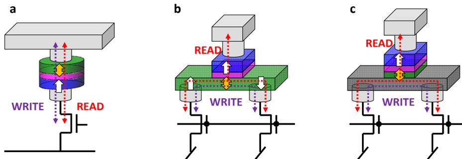
Fig. 1: Three kinds of spintronics memory devices addressed in this paper. **a**, Two-terminal spin-transfer torque (STT) switching device. **b**, Three-terminal domain wall (DW) motion device. **c**, Three-terminal spin-orbit torque (SOT) switching device.
