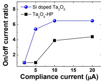
Fig. 6. On/off current ratios as a function of CC for Si-doped Ta<sub>2</sub>O<sub>5</sub> and Ta<sub>2</sub>O<sub>5</sub>-HP cells.
