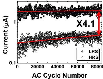
Fig. 7. AC endurance characteristics of Si-doped Ta<sub>2</sub>O<sub>5</sub> stack.
