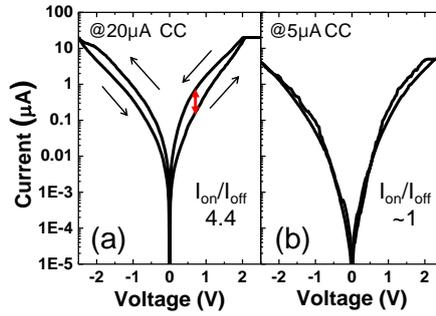
Fig. 4. The switching results after the fifth I-V sweeps for Ta<sub>2</sub>O<sub>5</sub>-HP with compliance current (CC). (a) 20μA CC, (b) 5μA CC. On/off current ratio was measured at 0.7V.
