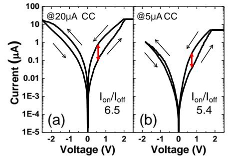
Fig. 5. The switching results after the fifth I-V sweeps for Si-doped (2.4% atomic percent) Ta<sub>2</sub>O<sub>5</sub> with CC. (a) 20μA CC, (b) 5μA CC.
