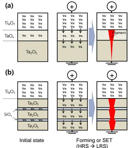
Fig. 11. Switching mechanism (a) Ta<sub>2</sub>O<sub>5</sub>-HP resistor, (b) Si doped Ta<sub>2</sub>O<sub>5</sub> resistor.
