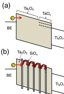
Fig. 9. Schematic band diagrams of (a) Ta<sub>2</sub>O<sub>5</sub>-HP and (b) Si-doped Ta<sub>2</sub>O<sub>5</sub> stack in HRS.
