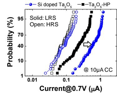
Fig. 10. HRS and LRS currents of Si doped Ta<sub>2</sub>O<sub>5</sub> and Ta<sub>2</sub>O<sub>5</sub>-HP cells.
