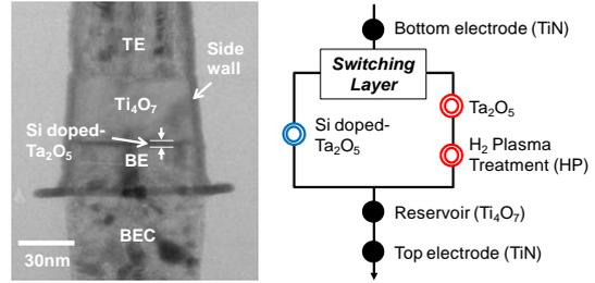
Fig. 2. (a) Crosssection TEM image of the fabricated ReRAM structure and (b) process flow. The bottom electrode contact (BEC) size is 50 nm
