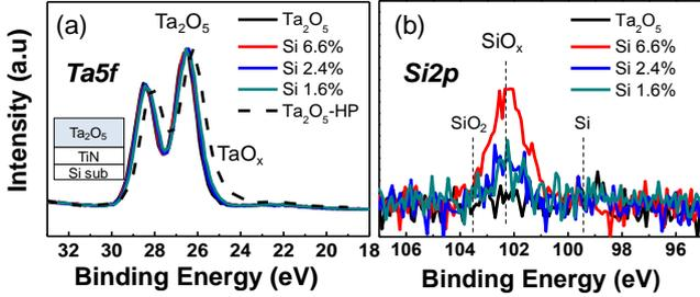
Fig. 3. XPS spectra of Ta<sub>2</sub>O<sub>5</sub>, Si-doped Ta<sub>2</sub>O<sub>5</sub>, and Ta<sub>2</sub>O<sub>5</sub>-HP.
