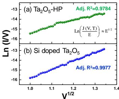
Fig. 8. Linear fitting of HRS from 5<sup>th</sup> cycle of switching I-V. (a) Ta<sub>2</sub>O<sub>5</sub>-HP, (b) Si doped Ta<sub>2</sub>O<sub>5</sub>.
