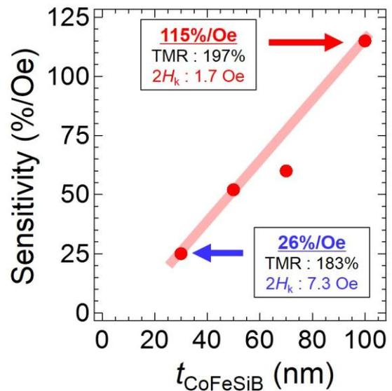
Fig. 4 CoFeSiB thickness dependence of sensitivity
