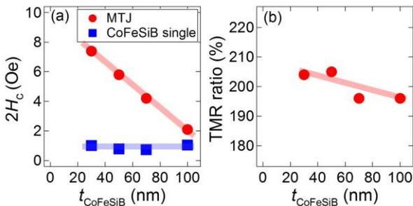
Fig. 1 CoFeSiB thickness ( $t_{\text{CoFeSiB}}$ ) dependence of (a) twice coercive field ( $2H_c$ ) of easy axis and (b) TMR ratio.
