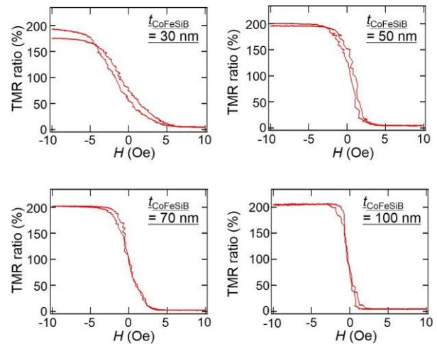
Fig. 3 Magnified vies of magneto-resistance curves in MTJ with each CoFeSiB thickness.
