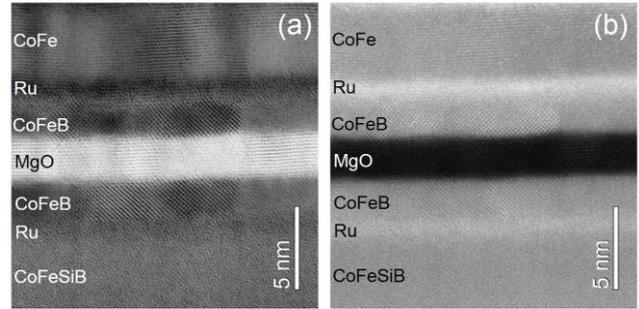
Fig. 2 STEM image (a) BF-STEM image, (b) HAADF-STEM image
