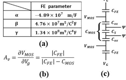
Fig. 2. (a) The parameters of PZT as the FE material in this work. (b) The express of voltage amplification by NC effect. (c) The effective circuits of FE gate stack of UTB-DG.
