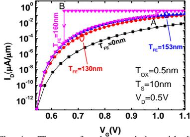
Fig. 4. The transfer characteristics with different  $T_{FE}$ . The hysteresis behavior is occurred with  $T_{FE}=160\text{nm}$ . Note that the  $T_{FE}=0\text{nm}$  indicates the control TFET without FE for reference.
