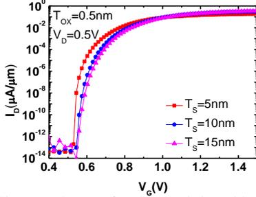
Fig. 7. The transfer characteristics with different  $T_S$ . The body thin-down is beneficial for extending steep SS region. Note that the  $T_{FE}$  is optimized thickness with steepest slope and non-hysteresis, i.e.  $C_{MOS} \sim |C_{FE}|$ .
