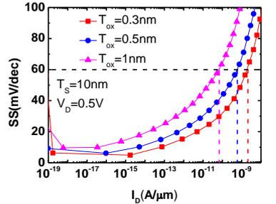
Fig. 12. The SS vs.  $I_D$  with different  $T_{OX}$ . It shows  $SS_{min} \sim 6\text{mV/dec}$  for 4 order with  $T_{OX} = 0.3\text{nm}$ .
