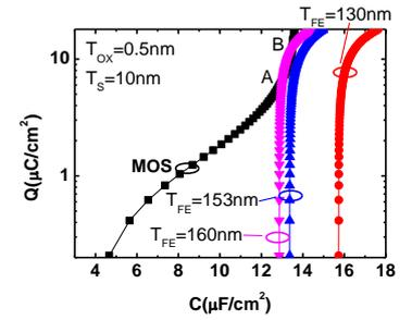
Fig. 3. The Q-C characteristics with different  $T_{FE}$ . The optimum condition is  $T_{FE}=153\text{nm}$  for minimum SS and non-hysteresis.
