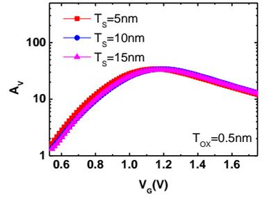
Fig. 9. The  $A_v$  with different  $T_S$ . The corresponding amplification of NC effect shows almost the same with different  $T_S$ .
