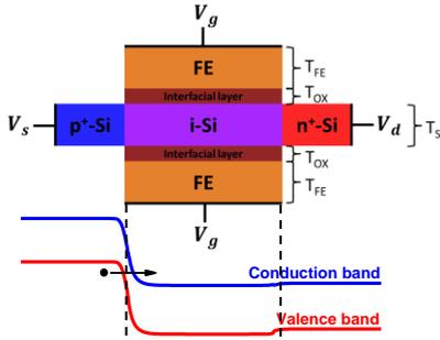
Fig. 1. The schematic diagram of UTB-DG-NC-TFET with  $L_g=40\text{nm}$ .  $T_{FE}$ ,  $T_S$ , and  $T_{OX}$  are the thickness of ferroelectric material, body and interfacial layer, respectively.
