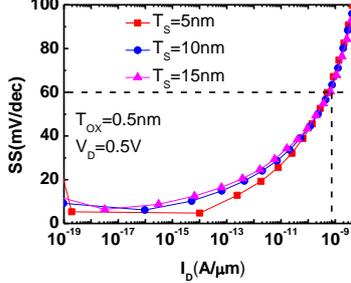
Fig. 8. The SS vs.  $I_D$  with different  $T_S$ . The  $SS_{min}$  ( $\sim 5\text{mV/dec}$ ) for  $\sim 5$  order is obtained with  $T_S = 5\text{nm}$
