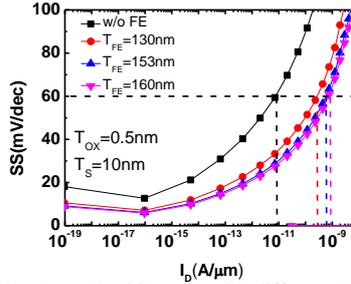
Fig. 5. The SS vs.  $I_D$  with different  $T_{FE}$ . The  $T_{FE}=153\text{nm}$  presents the non-hysteresis and steeper slope with denoting as optimized condition.
