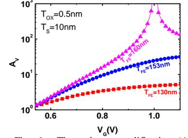
Fig. 6. The voltage amplification ( $A_v$ ) with different  $T_{FE}$ . The extracted peak  $A_v$  of the optimized condition shows that  $\sim 35$ .
