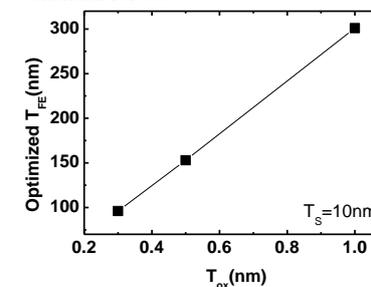
Fig. 14. The optimized  $T_{FE}$  vs  $T_{OX}$ . The optimized thickness of  $T_{FE}$  is decreasing with thinner  $T_{OX}$ . This indicates the possible PZT thickness for CMOS process integration with extreme thin  $T_{OX} \sim 0.3\text{nm}$  for non-hysteresis.
