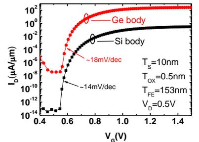
Fig. 15. The Ge TFET is beneficial for BTBT due to small bandgap, therefore, Ge UTB-DG-NC-TFET is a candidate for sub-10nm technology with steep slope ( $SS_{ave} \sim 18\text{mV/dec}$ ), high ON current ( $> 100\mu\text{A}/\mu\text{m}$ ), and  $< 0.2\text{V}$  switching voltage.
