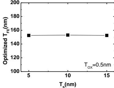
Fig. 10. The optimized  $T_{FE}$  vs.  $T_S$ . There is not significantly different in optimized  $T_{FE}$  with different  $T_S$ .
