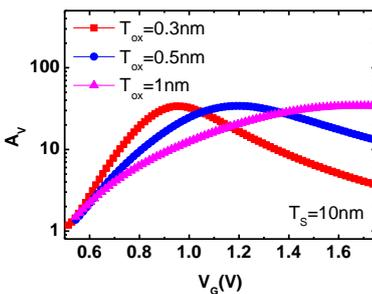
Fig. 13. The  $A_v$  with different  $T_{OX}$ . The negative shift in  $A_v$  peak with decreasing  $T_{OX}$  leads the steep slope in  $I_D$ - $V_G$
