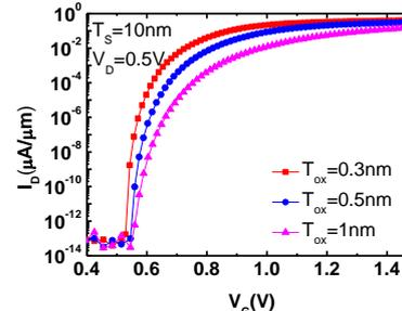
Fig. 11. The transfer characteristics with different  $T_{OX}$ . The thin-down interfacial layer is beneficial for SS.
