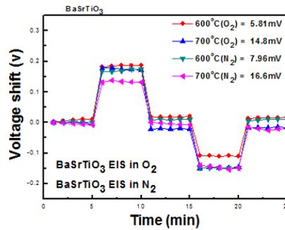
Fig. 4 Hysteresis of BaSrTiO<sub>3</sub> sensing membrane with various RTA temperatures in N<sub>2</sub> and O<sub>2</sub> ambient during the pH loop of 7→4→7→10→7 over a period of 25 minutes
