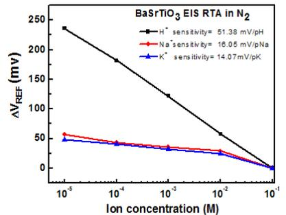
Fig. 6 The different ion sensitivity of BaSrTiO<sub>3</sub> sensing membrane annealed at 600°C in N<sub>2</sub> ambient
