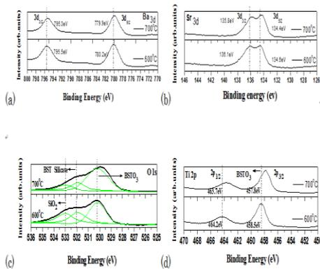
Fig. 1 XPS results of BaSrTiO<sub>3</sub> film (a) Ba 3d, (b) Sr 3d, (c) O 1s, (d) Ti 2p in O<sub>2</sub> ambient
