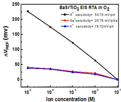
Fig.7 The different ion sensitivity of BaSrTiO<sub>3</sub> sensing membrane annealed at 600°C in O<sub>2</sub> ambient
