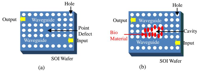
Fig. 1 Schematic structure of the proposed photonic crystal based biosensor (a) defect type and (b) cavity type.
