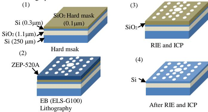
Fig. 4 Fabrication process.
