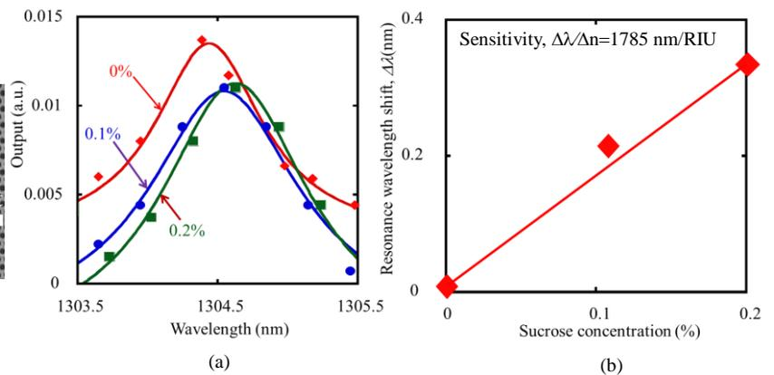
Fig. 7 Measured results of fabricated device (a) resonance peak shift with respect to sucrose concentration and (b) sucrose concentration versus resonance wavelength shift.
