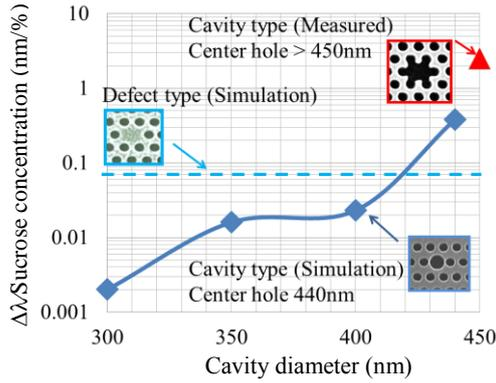
Fig. 3 Comparison of simulation and measured results at different cavity diameters. Defect type simulation results also include in this graph
