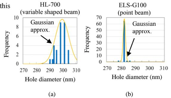
Fig. 5 Comparison of scattering of hole size fabricated by (a) HL-700 and (b) ELS-G100 lithography machines.
