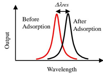
Fig. 2 Operation principle of the proposed device.
