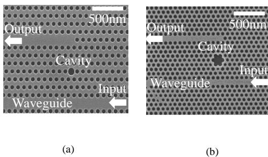
Fig. 6 Scanning electron micrograph of the fabricated device (a) normal cavity type and (b) abnormal cavity type (with larger diameter).
