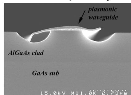
Fig. 2 SEM cross-sectional image of the under-etched plasmonic waveguide.
