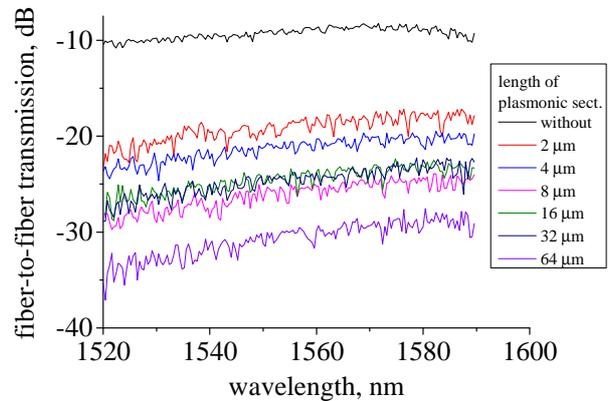
Fig. 5 Fiber-to-fiber transmission of the Si/SiO<sub>2</sub>/Si/Ti<sub>2</sub>O<sub>3</sub>/Co plasmonic waveguide integrated with a Si nanowire waveguides. The black line shows the transmission for a Si nanowire waveguide without a plasmonic section.
