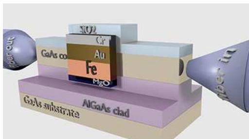
Fig. 1 Ferromagnetic plasmonic waveguide monolithically integrated with AlGaAs/GaAs optical waveguide. The transmission of light from input to output fiber is measured.
