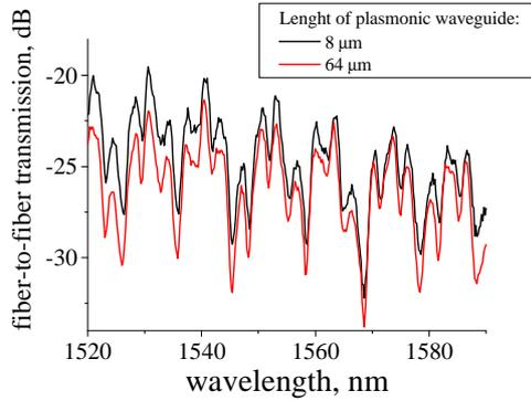
Fig. 3 Fiber-to-fiber transmission of the AlGaAs/MgO/Fe plasmonic structure embedded into the AlGaAs/GaAs optical waveguide.
