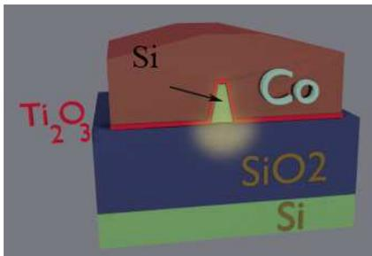
Fig. 4 Wedge-type Si/SiO<sub>2</sub>/Si/Ti<sub>2</sub>O<sub>3</sub>/Co plasmonic waveguide . The field distribution of plasmon is shown in yellow color.
