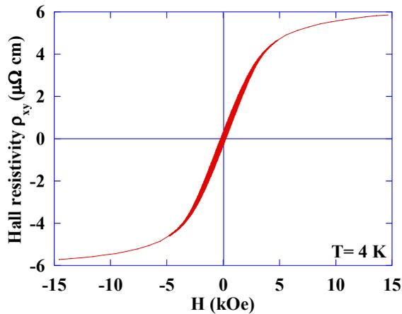
Fig. 3 Hall resistivity ( $\rho_{xy}$ ) of MCA films formed at  $300^\circ\text{C}$  as a function of the applied magnetic field ( $H$ ) measured at 4 K.
