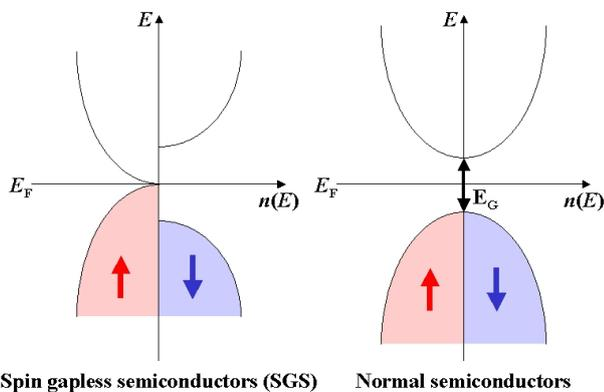
**Fig. 1** Typical density of states (DOS) of spin gapless semiconductors (SGS) (left figure). The DOS of normal semiconductors with bandgap of  $E_G$  is also shown as comparison (right figure).
