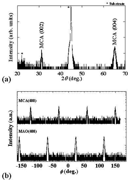
Fig. 2 (a) Out-of-plane and (b) in-plane XRD patterns for MCA films on MAO substrates ( $T_g=550^\circ\text{C}$ ).
