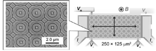
Fig. 2 Schematic diagram for the Hall bar sample used in the present work. The left and right panels show the SEM micrograph and the Hall bar device of MLA, made of InGaAs/InAlAs quantum well, used in the measurement. We have 5,408 rings in the actual Hall bar.
