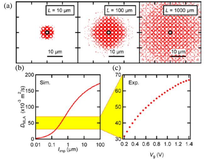
Fig. 3 (a) Snapshots of classical diffusion of Boltzmannian electrons in MLA with  $l_{imp} = 1.0 \mu\text{m}$ . (b) The  $D_{MLA}$  values by the chaotic billiard simulation as a function of  $l_{imp}$ . Here, we use  $v_F = 8.51 \times 10^5 \text{m/s}$ . (c) The experimental values of  $D_{MLA}$  as a function of  $V_g$ .
