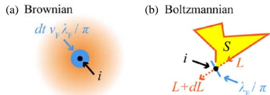
Fig. 1 Schematic pictures for the concept of *return*. (a) Brownian picture. (b) Boltzmannian picture. Black point  $i$  in (a) and (b) shows the initial point at  $t=0$  (origin). The blue area in (a) represents  $\delta S$  and the blue line in (b) shows the *judge length* for the *returning* criterion. We also show the enclosed area  $S$  in the Boltzmannian picture (b).
