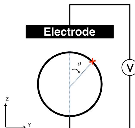
Fig. 1 A structural model of a CNT under an electric field. A cross indicates the position of the defects. The angle ( $\theta$ ) denotes the mutual angle of the defect with respect to the electrode.
