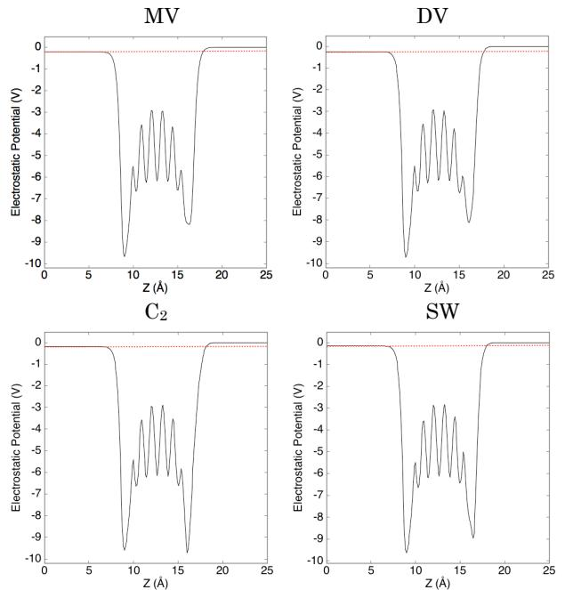
Fig 2 Plane averaged electrostatic potentials of CNTs with monovacancy (MV), divacancy (DV),  $C_2$  adatom ( $C_2$ ), and Stone–Wales defect (SW) normal to the z-direction under a zero electric field. The electrode is on the right end of the panel. Horizontal dotted lines denote vacuum level at the left end of the unit cell.
