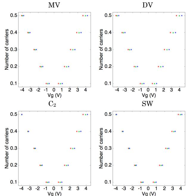
Fig 3 The number of accumulated carriers in CNT as a function of the external electric field. Circles, triangles, and squares denote the CNTs with the defects of which mutual angles are 0, 90, and 180 degree, respectively.
