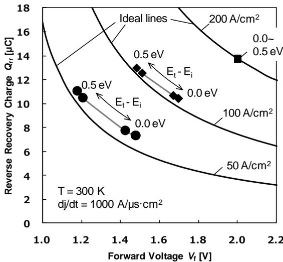
Fig. 3 The relationship between  $V_f$  and  $Q_{rr}$  for various values of  $J$ .
