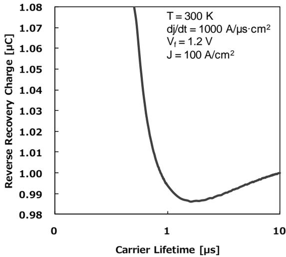
Fig. 2 The relationship between  $Q_{rr}$  and  $\tau_i$  for  $V_f = 1.2$  V and  $J = 100$  A/cm<sup>2</sup>.
