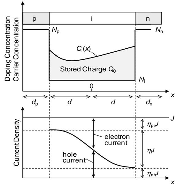
Fig. 1 Schematic of the pin diode with the doping distribution, excess carrier concentration, and current density.
