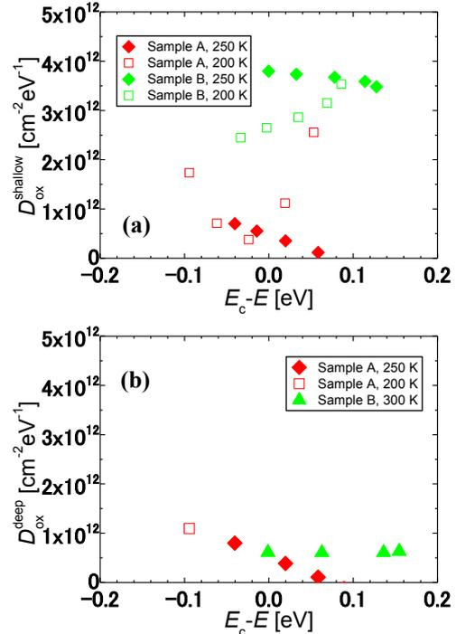
Fig. 5 (a)  $D_{\text{ox}}^{\text{shallow}}$  and (b)  $D_{\text{ox}}^{\text{deep}}$  of the samples estimated by the measurements at different temperatures.
