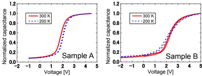
Fig. 2 1 MHz bidirectional  $C$ - $V$  characteristics of two kinds of SiC MOS capacitors A and B.
