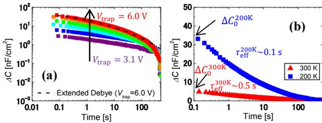
Fig. 3  $C$ - $t$  characteristics of sample B, (a) with various  $V_{\text{trap}}$  at 200 K, and (b) at different temperatures with  $V_{\text{trap}} = 6.0$  V.
