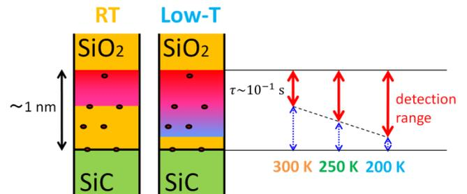
**Fig. 1** Schematic of oxide trap detection range of spatial distance from SiO<sub>2</sub>/SiC interface at various temperatures. The distance from the interface indicated in the figure is approximately estimated by taking account of the tunneling mass of electrons and eq.(3).
