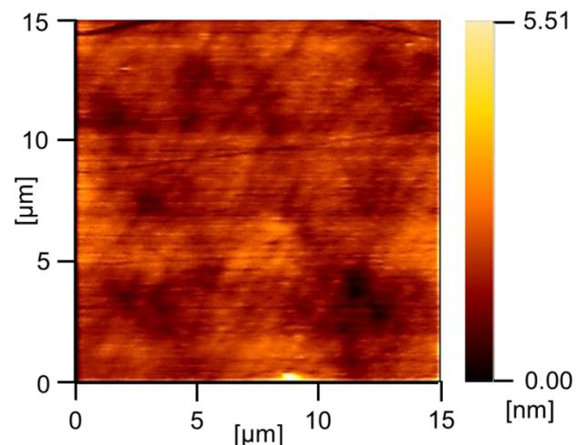
Fig. 5 AFM image of the SiC epitaxial layer surface before bonding.
