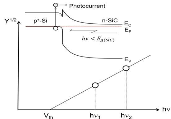
Fig. 2 Energy band diagram of the p<sup>+</sup>-Si/n-SiC heterojunction and a PR spectra.
