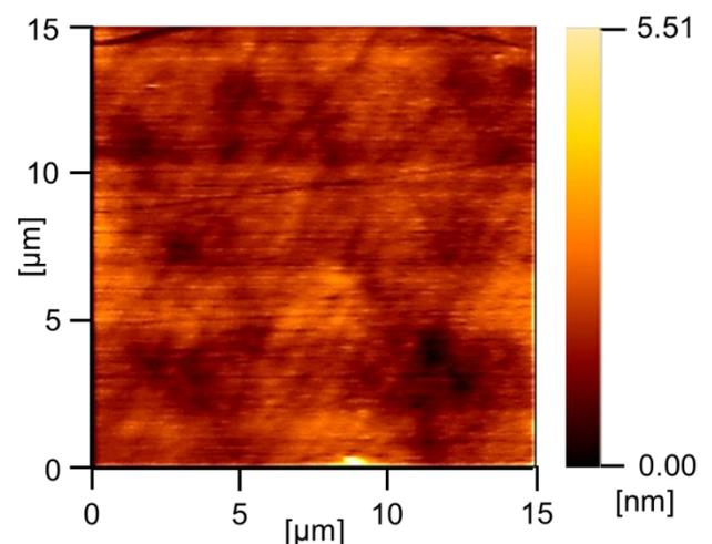
Fig. 5 AFM image of the SiC epitaxial layer surface before bonding.
