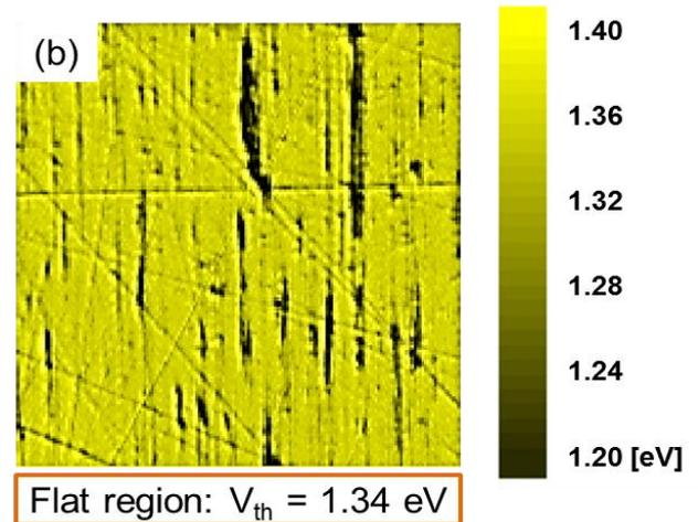
Fig. 4 (a)  $Y$  ( $\lambda = 516$  nm) and (b)  $V_{th}$  maps of the  $p^+$ -Si/n-SiC heterojunction by SIPM.
