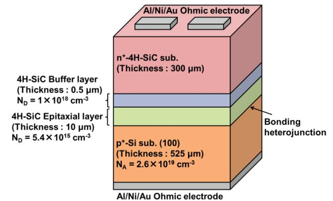
Fig. 1 Device structure.
