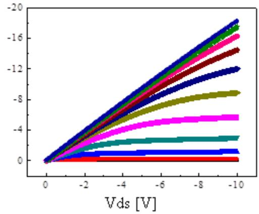
Fig.4  $I_{DS}-V_{DS}$  characteristics of trench-channel diamond MOSFET
