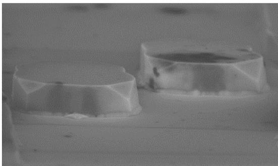
Fig.4 The inside of a trench after un-doped layer is re-grown (taken by SEM)
