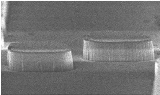
Fig.3 The inside of a trench before the un-doped layer is re-grown (taken by SEM)
