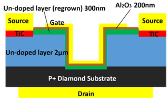
Fig.5. Vertical-shaped MOSFET with  $\text{Al}_2\text{O}_3$  oxide
