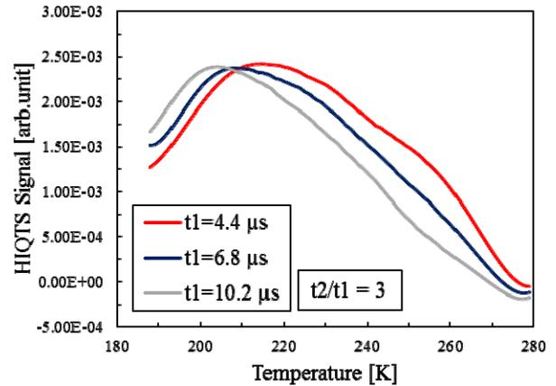
Fig. 3 HIQTS spectra extracted from charge transient signal by applying rate window method
