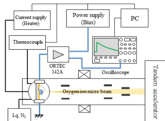
Fig. 1 Schematic diagram of HIQTS system based on 3MV tandem accelerator
