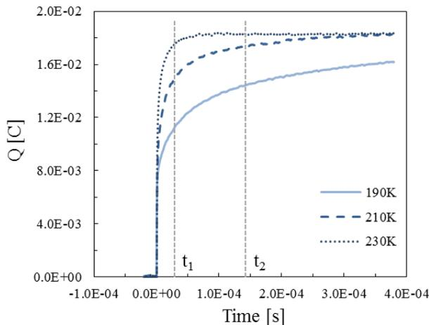
Fig. 2 HIQTS signals obtained at temperature of 190K, 210K, and 230K
