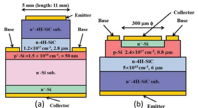
Fig. 1. A schematic cross section of 4H-SiC/Si HBT structures fabricated by the surface activated bonding.
