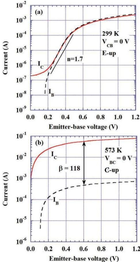
Fig. 2.  $I_B$ - $V_{EB}$  and  $I_C$ - $V_{EB}$  characteristics with  $V_{CB}$  of 0 V measured for the SiC/Si HBT at 299 (a) and 573 K (b), respectively. The dependencies of  $\alpha$  on the ambient temperature for the E-up (a) and C-up (b) structures, respectively.
