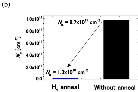
Fig. 3 (a) Oxide thickness dependence of  $V_{fb}$  for the MOS capacitors with or without 1%-H<sub>2</sub> annealing. (b) Estimated  $N_{it}$  from the slope.  $N_{it}$  is significantly suppressed by 1%-H<sub>2</sub> annealing.
