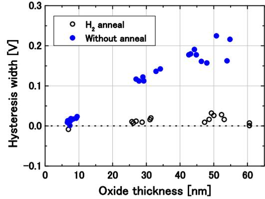
Fig. 4 Oxide thickness dependence of hysteresis width of C-V curves defined at  $V_G = V_{FB}$  for the MOS capacitors with and without 1%-H<sub>2</sub> annealing. Positive values indicate clockwise hysteresis and negative values indicate counter-clockwise.
