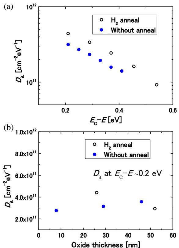
Fig. 2 (a)  $D_{it}$  of the MOS capacitors (CET $\sim 30$ nm) with or without 1%-H<sub>2</sub> annealing, as a function of energy level below the conduction band of SiC.  $D_{it}$  was measured by conductance method at room temperature. (b) Oxide thickness dependence of  $D_{it}$  at  $E_C - E \sim 0.2$  eV for the capacitors with or without 1%-H<sub>2</sub> annealing.
