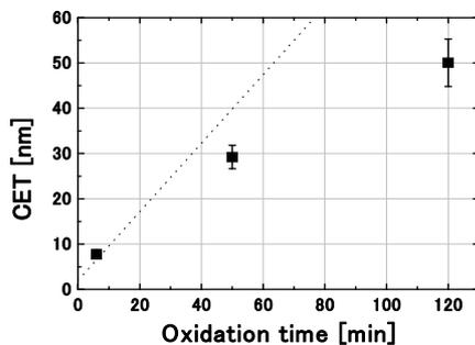
Fig. 1 Relationship between oxidation time and thermal oxide thickness grown at 1250°C in 1-atm-O<sub>2</sub>. The vertical axis is the capacitance equivalent oxide thickness (CET). Dotted line is corresponding to the interface-reaction-limited growth case estimated from [1].
