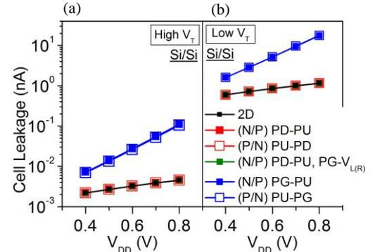
Fig. 6. 6T SRAM cell leakage comparison of (a) high  $V_T$  and (b) low  $V_T$  design for 2D and 3D Si/Si SRAM scenarios.
