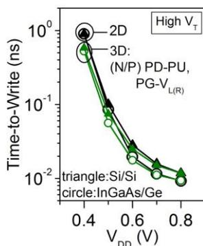
Fig. 11. Cell Time-to-Write of InGaAs/Ge and Si/Si SRAMs for 2D and 3D SRAM scenarios.
