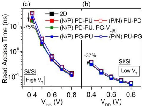
Fig. 7. Cell Read access time of (a) high  $V_T$  and (b) low  $V_T$  design for 2D and 3D Si/Si SRAM scenarios.
