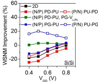
Fig. 5. WSNM improvement of high  $V_T$  designs over low  $V_T$  counterparts for 2D and 3D Si/Si SRAM scenarios.
