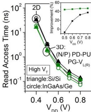
Fig. 10. Cell Read access time of InGaAs/Ge and Si/Si SRAMs for 2D and 3D SRAM scenarios. The inset shows the Read access time improvement of InGaAs/Ge over Si/Si counterparts for 2D and 3D results.
