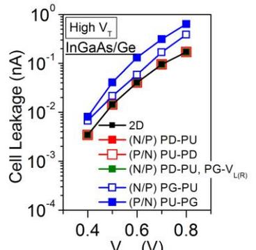
Fig. 13. Cell leakage of high  $V_T$  InGaAs/Ge SRAM for 2D and 3D scenarios.
