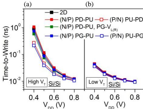
Fig. 8. Cell Time-to-Write of (a) high  $V_T$  and (b) low  $V_T$  design for 2D and 3D Si/Si SRAM scenarios.
