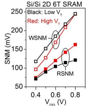
Fig. 3. RSNM and WSNM of Si/Si 2D 6T SRAMs with high/low  $V_T$  design versus  $V_{DD}$ .
