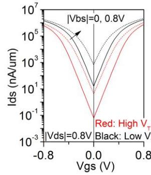
Fig. 2.  $I_{ds}$ - $V_{gs}$  curves of UTB SOI devices with high/low  $V_T$  design under zero and forward body-to-source bias.
