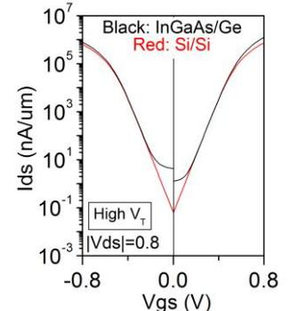
Fig. 9.  $I_{ds}$ - $V_{gs}$  curves of UTB InGaAs-OI/Ge-OI and Si/Si with  $V_T = 0.4V$ .
