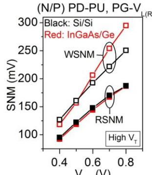
Fig. 12. RSNM and WSNM of 3D (N/P) PD-PU, PG- $V_{L(R)}$  Si/Si and InGaAs/Ge 6T SRAM.
