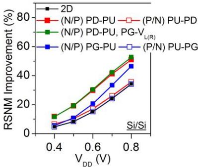
Fig. 4. RSNM improvement of high  $V_T$  designs over low  $V_T$  counterparts for 2D and 3D Si/Si SRAM scenarios.
