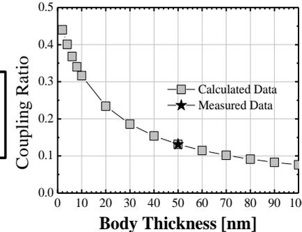
Fig. 6 Body thickness dependence on coupling ratio between  $\Delta V_T$  for G1 and G2.
