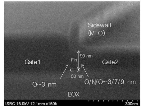
Fig. 1 Structure of the asymmetric dual-gate device.
