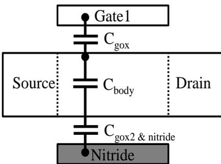
Fig. 5 Simple capacitance network model in the device.
