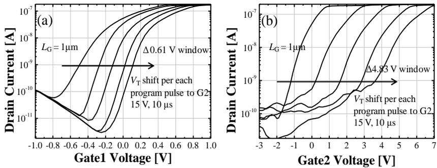
Fig. 4 Measured (a)  $I_D$ - $V_{G1}$  curves and (b)  $I_D$ - $V_{G2}$  curves of the device with  $V_D = 1$  V as a function of programming pulses.
