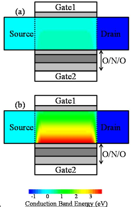
Fig. 7 Contours of conduction band energy with  $V_G = 0$  V and  $V_D = 1$  V when nitride layer is (a) neutral and (b) negatively charged.
