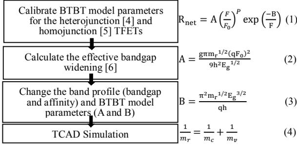
Fig. 2. Methodology used in this work.  $R_{\text{net}}$  is the BTBT generation rate and  $P=2$ .  $F$  is the electric field and  $F_0=1\text{V/cm}$ .  $g$  is the degeneracy factor and  $E_g$  is the bandgap.  $m_v$  and  $m_c$  are the effective mass of conduction band and valence band.
