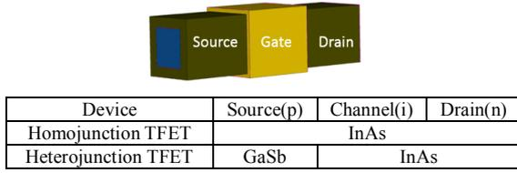
Fig. 1. Schematic sketch of a GAA structure. The source doping is  $4 \times 10^{19} \text{ cm}^{-3}$ , while the drain doping is  $6 \times 10^{17} \text{ cm}^{-3}$  to suppress the ambipolar behavior. The supply voltage is 0.3V.
