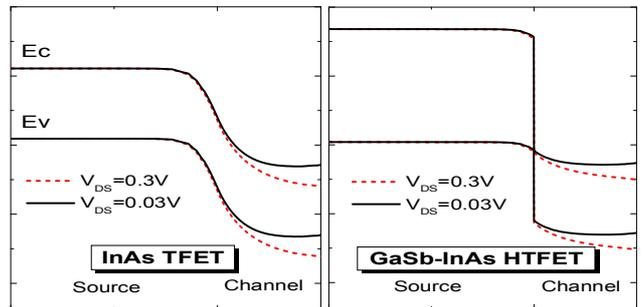
Fig. 8. Band diagram of the source-channel junction for InAs TFET and GaSb-InAs HTFET with  $V_{\text{DS}}=0.3\text{V}$  and  $V_{\text{DS}}=0.03\text{V}$  when the diameter= $10\text{nm}$  and the gate length= $10\text{nm}$ .
