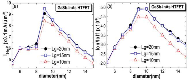
Fig. 6.  $I_{60\text{mV}}$  and  $I_{\text{on}}/I_{\text{off}}$  versus diameter for GaSb-InAs HTFET with various  $L_g$  and  $EOT=0.65\text{nm}$ .
