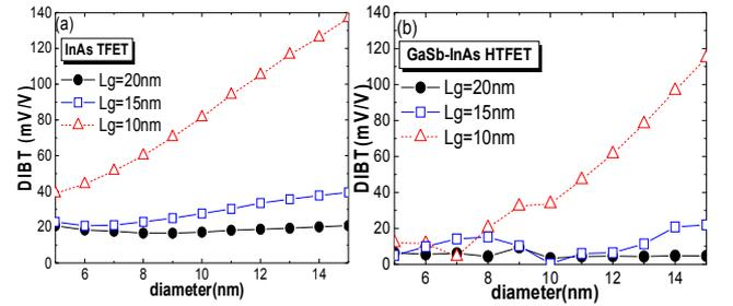
Fig. 7. DIBT versus diameter for InAs TFET and GaSb-InAs HTFET. DIBT is defined as the  $V_t$  reduction (constant current= $10^{-1} \text{ mA}/\mu\text{m}^2$  [7]) as  $V_{\text{DS}}$  increases from 30mV to 0.3V.
