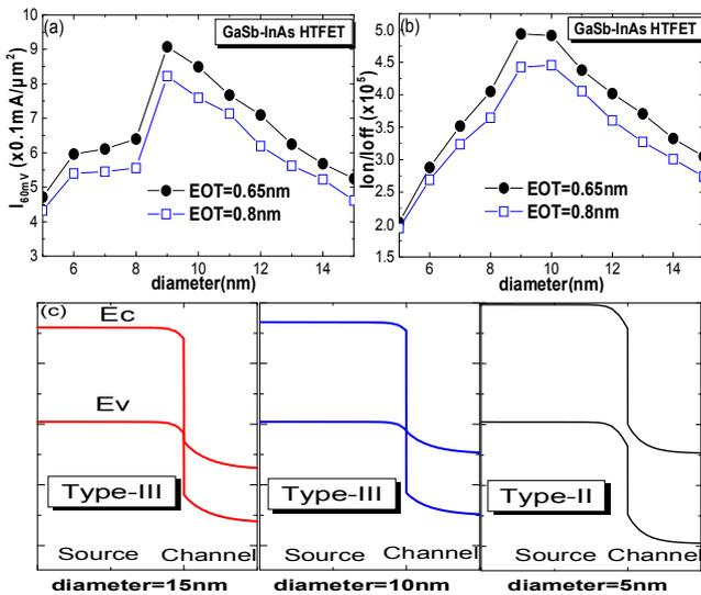
Fig. 4. (a)(b)  $I_{60\text{mV}}$  and  $I_{\text{on}}/I_{\text{off}}$  versus diameter for GaSb-InAs HTFET with various EOT and  $L_g=20\text{nm}$ . (c) The band alignment changes from type-III to type-II with decreasing diameter.
