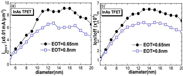
Fig. 3.  $I_{60\text{mV}}$  and  $I_{\text{on}}/I_{\text{off}}$  versus diameter for InAs TFET with various EOT and  $L_g=20\text{nm}$ .
