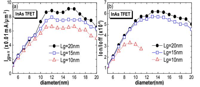
Fig. 5.  $I_{60\text{mV}}$  and  $I_{\text{on}}/I_{\text{off}}$  versus diameter for InAs TFET with various  $L_g$  and  $EOT=0.65\text{nm}$ .
