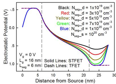
Fig. 7 Electrostatic potential distributions 0.625nm from channel surface.  $V_g = 0$  V.
