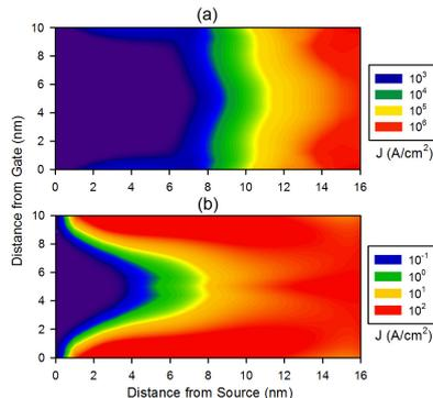
Fig. 3 On-state electron current density distributions: (a) TFET and (b) STFET.
