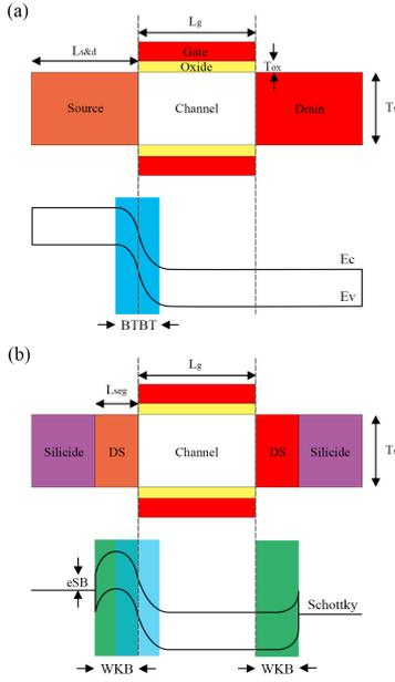
Fig. 1 Schematic structures and energy band diagrams of (a) TFET and (b) STFET.
