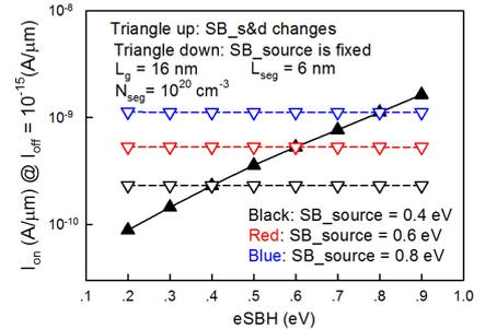
Fig. 9  $I_{on}$  versus  $eSBH$  for STFET with fixed  $SBH$  at source side.  $V_{dd} = 0.5$  V, and  $I_{off}$  is fixed at  $10^{-15}$  A/μm.
