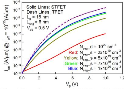
Fig. 4 Transfer curves of TFET and STFET with different  $N_{seg}$  at source side.  $V_{dd} = 0.5$  V, and  $I_{off}$  is fixed at  $10^{-15}$  A/μm.
