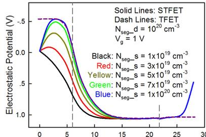
Fig. 5 Electrostatic potential distributions 0.625nm from channel surface.  $V_g = 1$  V.
