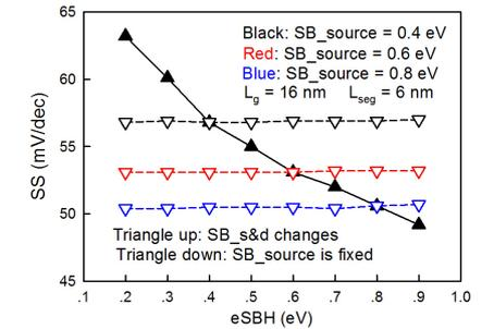
Fig. 10  $SS$  versus  $eSBH$  for STFET with fixed  $SBH$  at source side.
