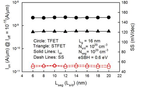
Fig. 8  $I_{on}$  and  $SS$  versus  $L_{seg}$  ( $L_{s/d}$ ) for TFET and STFET.  $V_{dd} = 0.5$  V, and  $I_{off}$  is fixed at  $10^{-15}$  A/μm.
