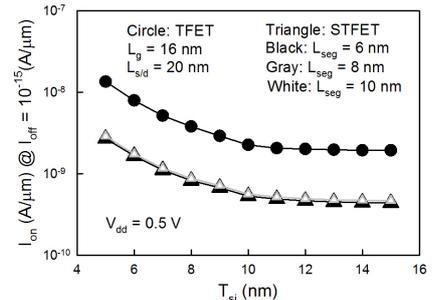
Fig. 11  $I_{on}$  versus  $T_{si}$  for TFET and STFET.  $V_{dd} = 0.5$  V, and  $I_{off}$  is fixed at  $10^{-15}$  A/μm.
