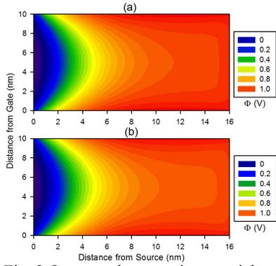
Fig. 2 On-state electrostatic potential distributions: (a) TFET and (b) STFET.
