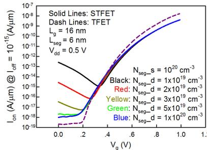
Fig. 6 Transfer curves of TFET and STFET with different  $N_{seg}$  at drain side.  $V_{dd} = 0.5$  V, and  $GWF$  for STFET is 4.265 eV.
