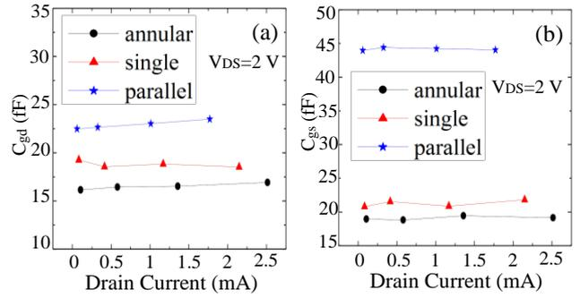
Fig. 5 Extracted (a)  $C_{gd}$  and (b)  $C_{gs}$  of poly-Si TFTs with different layout structures.
