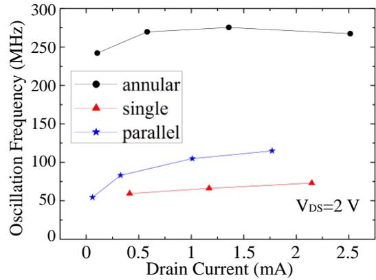
Fig. 6  $f_{max}$  of poly-Si TFTs with different layout structures.
