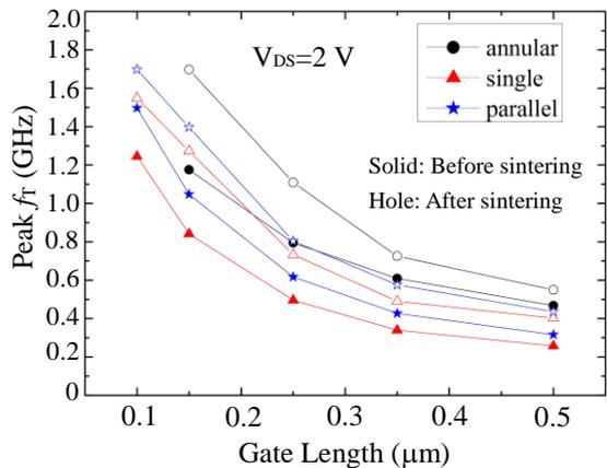
Fig. 8 Nonsintered and sintered peak  $f_t$  of poly-Si TFTs with different layout structures.
