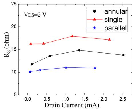
Fig. 7 Extracted  $R_g$  of poly-Si TFTs with different layout structures.
