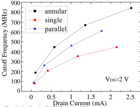
Fig. 3  $f_t$  of poly-Si TFTs with different layout structures.
