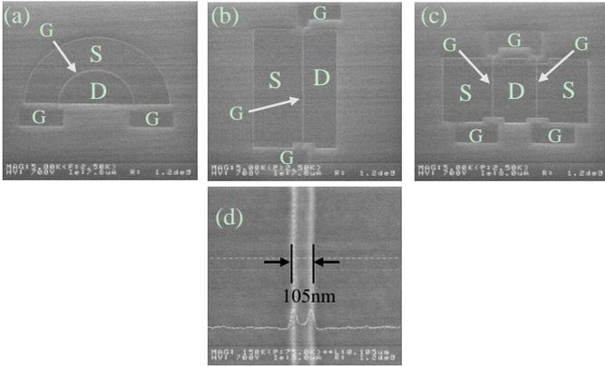
Fig. 1 Top-view SEM image of (a) annular, (b) single, (c) parallel, and (d) active region of poly-Si TFT with  $L = 105 \text{ nm}$ .
