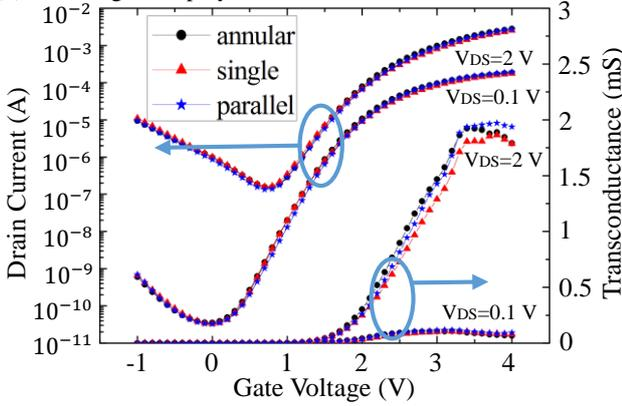
Fig. 2 The  $I_{DS} - V_{GS}$  transfer curves with different layout structures.
