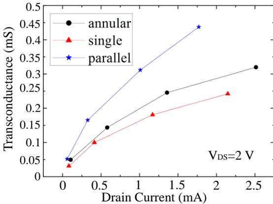
Fig. 4 Extracted transconductance of poly-Si TFTs with different layout structures.
