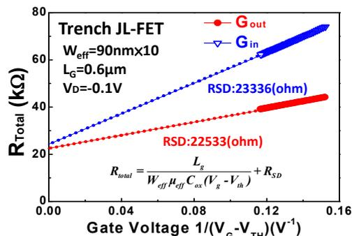
Fig. 6.  $R_{total}$  for  $G_{out}$  and  $G_{in}$  trench JL-FETs with  $L_G = 0.6 \mu\text{m}$ .
