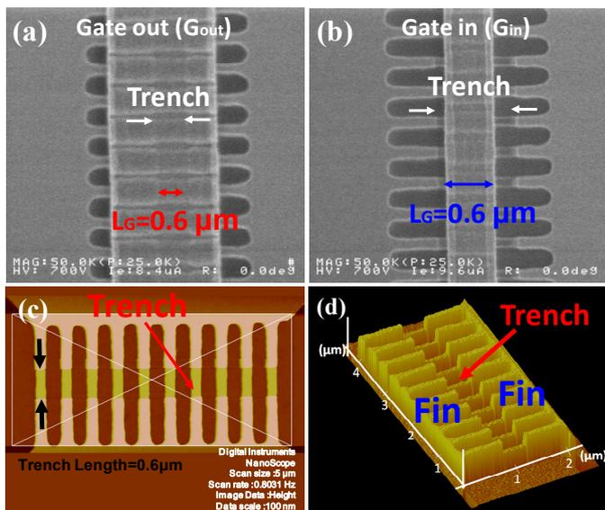
Fig. 2. Top-view SEM image of trench JL-FET for (a)  $G_{out}$  and (b)  $G_{in}$  structures with effective  $L_G = 0.6 \mu\text{m}$ .  $G_{out}$  device controls more active region.  $G_{in}$  device has small device area. (c) & (d) are AFM images of active channel region of trench JL-FET with ten NWs.
