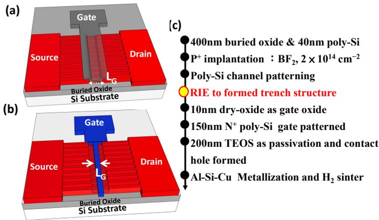
Fig. 1. (a)  $G_{out}$  structure and (b)  $G_{in}$  structure trench JL-FET devices. (c) Process flow chart of the these devices fabrication.
