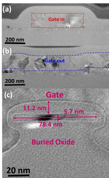
Fig. 3. TEM images for (a)  $G_{in}$  and (b)  $G_{out}$  structure trench JL-FET with effective  $L_G = 0.6 \mu\text{m}$ .  $G_{out}$  device controls more active region.  $G_{in}$  device has small device area. (c) TEM image along gate direction to form the  $\Omega$ -gate structure.  $W_{eff} = (78.4 \text{ nm} + 5.7 \text{ nm} \times 2) \times 10 = 90 \text{ nm} \times 10$
