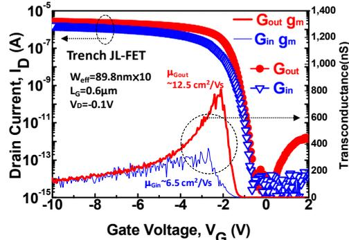
Fig. 5.  $I_D$ - $V_G$  curves of  $G_{out}$  and  $G_{in}$  trench JL-FETs with  $L_G = 0.6 \mu\text{m}$ . The  $G_{out}$  device has a higher  $g_m$  and  $\mu$ , owing to more channel control area (Fig. 2a) and the benefit of effective raised source/drain.
