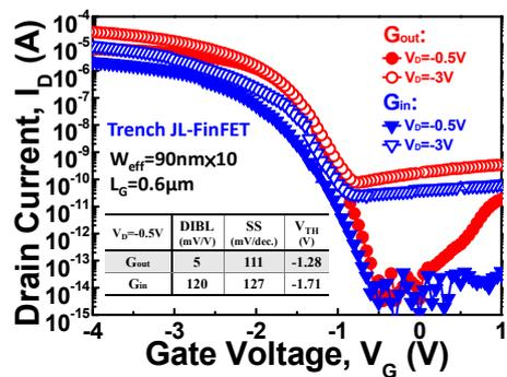
Fig. 4. Comparison of the  $I_D$ - $V_G$  curves of  $G_{out}$  and  $G_{in}$  NWs trench JL-FET with  $L_G = 0.6 \mu\text{m}$  at  $V_D = -0.5V$  and  $-3V$ . The  $G_{out}$  device has higher  $I_{on}$  and  $I_{off}$  than that of  $G_{in}$  device.
