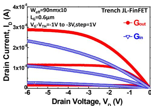
Fig. 7.  $I_D$ - $V_D$  curves of  $G_{out}$  and  $G_{in}$  trench JL-FET with  $L_G = 0.6 \mu\text{m}$ .
