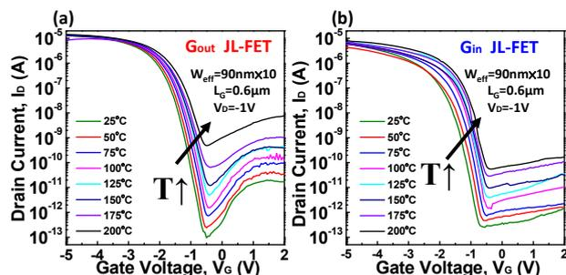
Fig. 8. Temperature dependence on  $I_D$ - $V_G$  curves of  $G_{out}$  and  $G_{in}$  devices.
