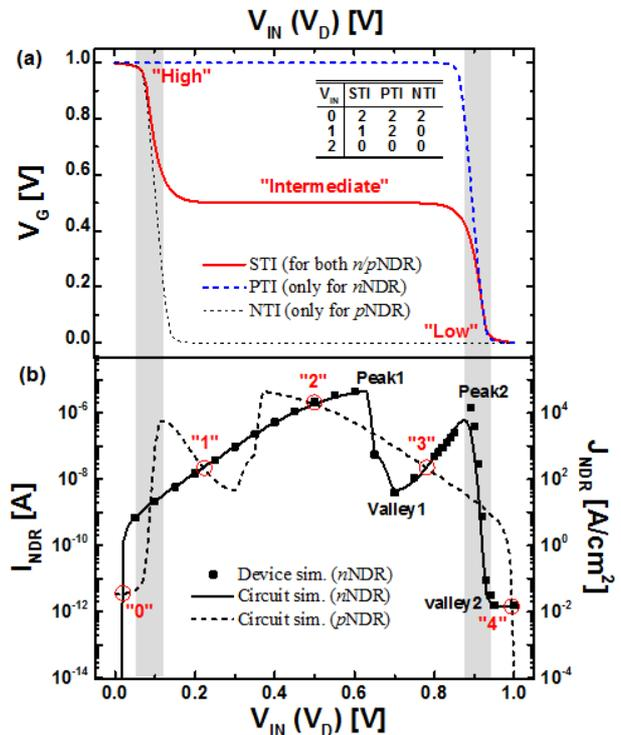
Fig. 2 (a) Simulated voltage transfer curve (VTC) of CMOS STI/PTI/NTI (b) complementary NDR characteristics of *n*NDR and *p*NDR based on Fig. 1(a)
