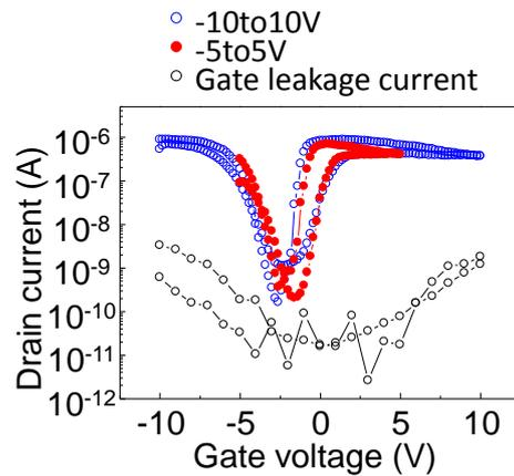
Fig. 4  $I_D$ - $V_G$  and gate leakage current of the FET at the drain voltage of 1 V.
