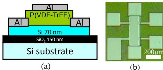
Fig. 1 Schematic image of cross sectional view, (a), and the optical microscope image, (b), of the FET.
