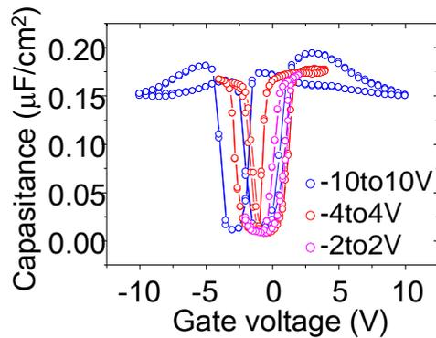
Fig. 3 C-V characteristics of Al/P(VDF-TrFE)/Si MFS structure at the measurement frequency of voltage of 1 kHz.
